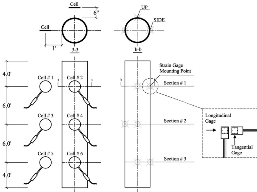
**Figure 4.35 Detailed view of instrumentation for 18-inch diameter HDPE drainage pipe (not to scale)**
