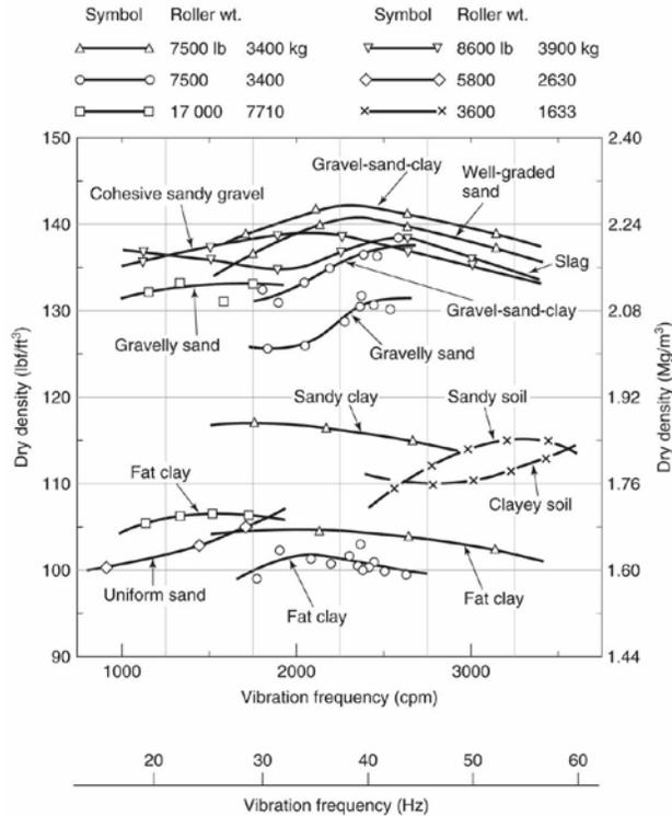
**Figure 2.2 Effect of vibration frequency on compaction by smooth-drum vibratory rollers (after several sources as cited by Selig and Yoo 1977)**
