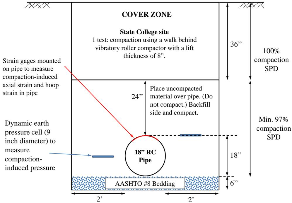
**Figure 3.13 Cross-sectional view of trench and instrumentation for 18-inch diameter reinforced concrete pipe (not to scale)**
