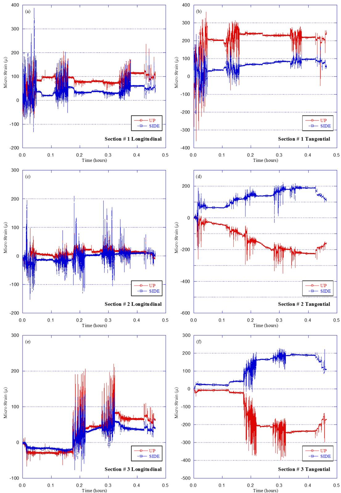
**Figure 4.20** Strains along pipe versus time for Test HB-7 (SDR-35 pipe in 2A aggregates)
