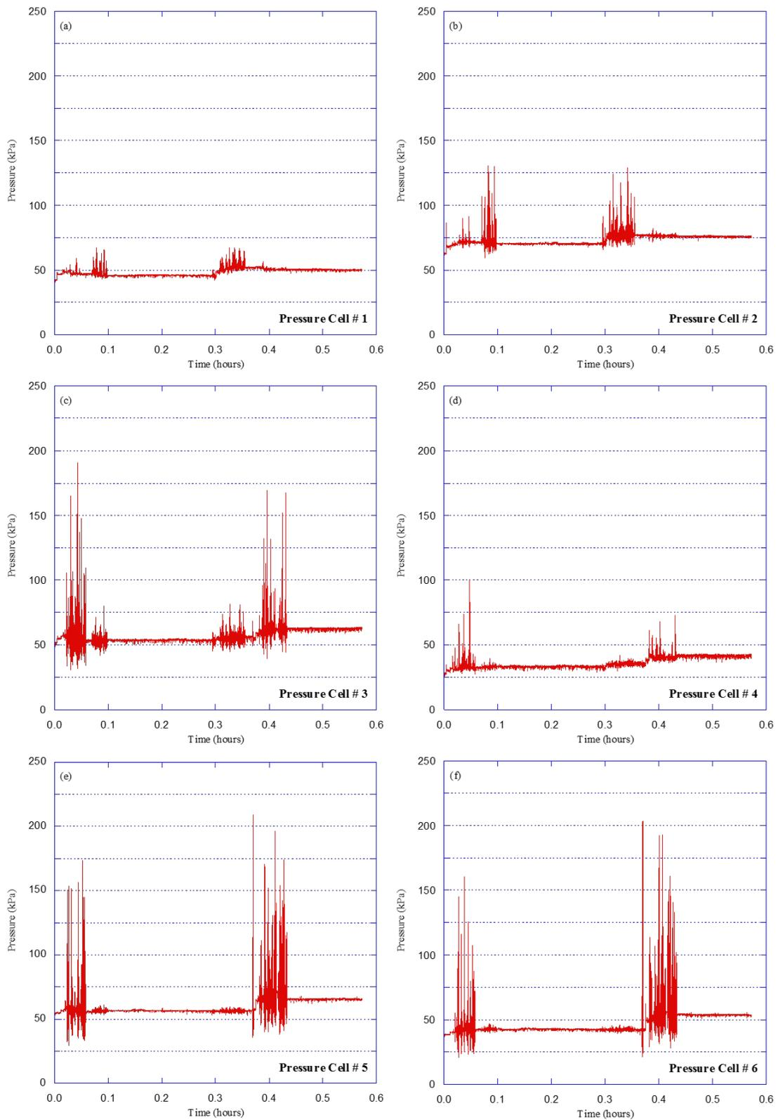
**Figure 4.28 Downward earth pressures versus time for Test HB-10 (reinforced concrete pipe)**
