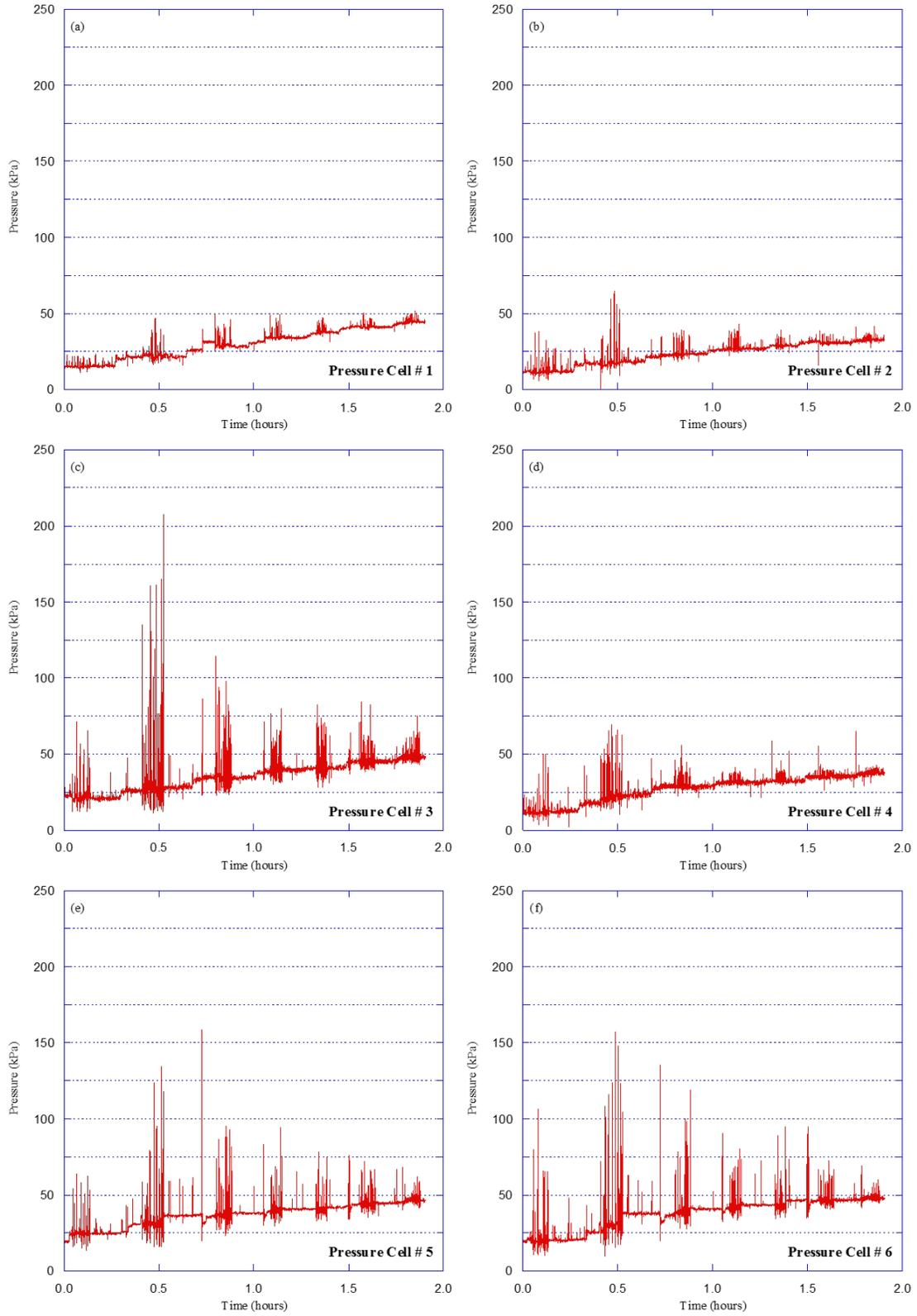
**Figure 3.11 Downward earth pressures versus time for Test SC-2 (SDR-35 pipe in 2A aggregates)**
