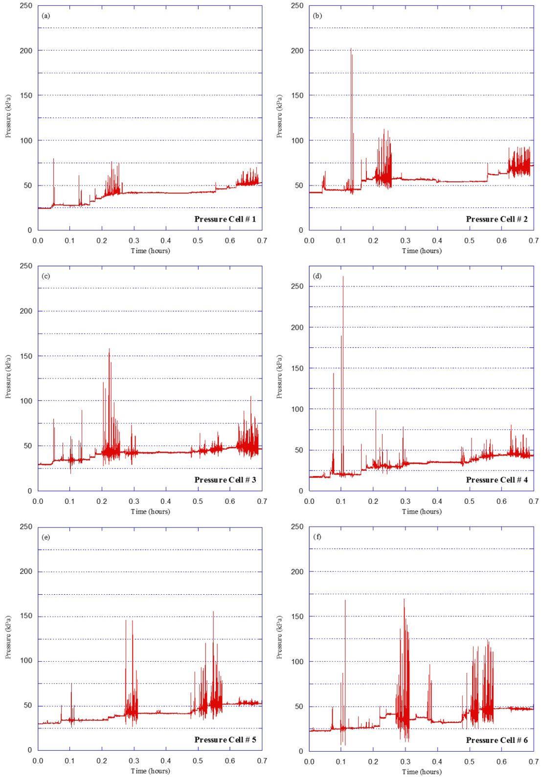
**Figure 4.37 Downward earth pressures versus time for Test HB-13 (HDPE drainage pipe)**
