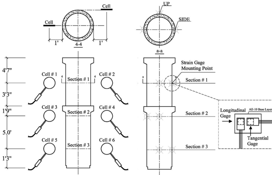
**Figure 3.14 Detailed view of instrumentation for 18-inch diameter reinforced concrete pipe (not to scale)**
