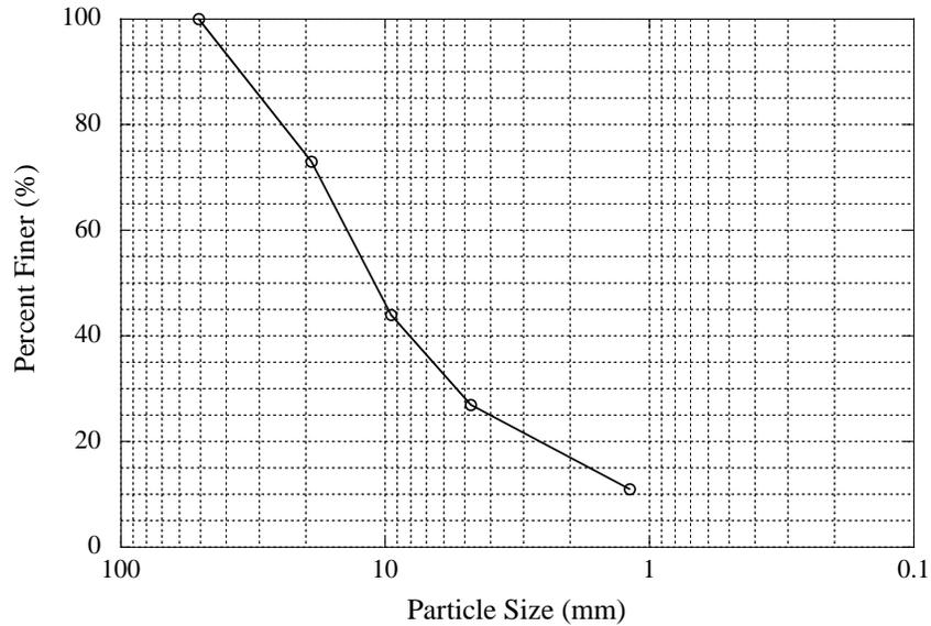
**Figure 1.3 Grain size distribution of 2A aggregates**
