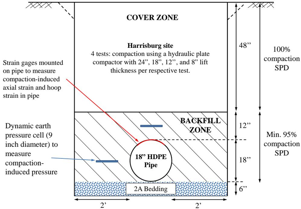
**Figure 4.34 Cross-sectional view of trench and instrumentation for 18-inch diameter HDPE drainage pipe (not to scale)**
