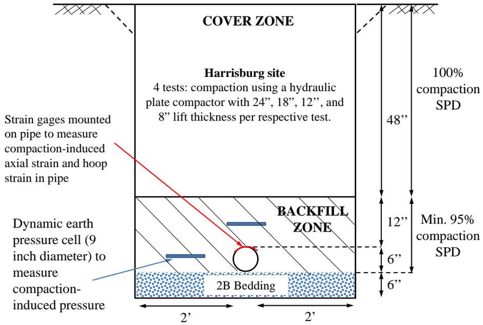
**Figure 4.12 Cross-sectional view of trench and instrumentation for 6-inch diameter SDR-35 pipe in 2A aggregates (not to scale)**
