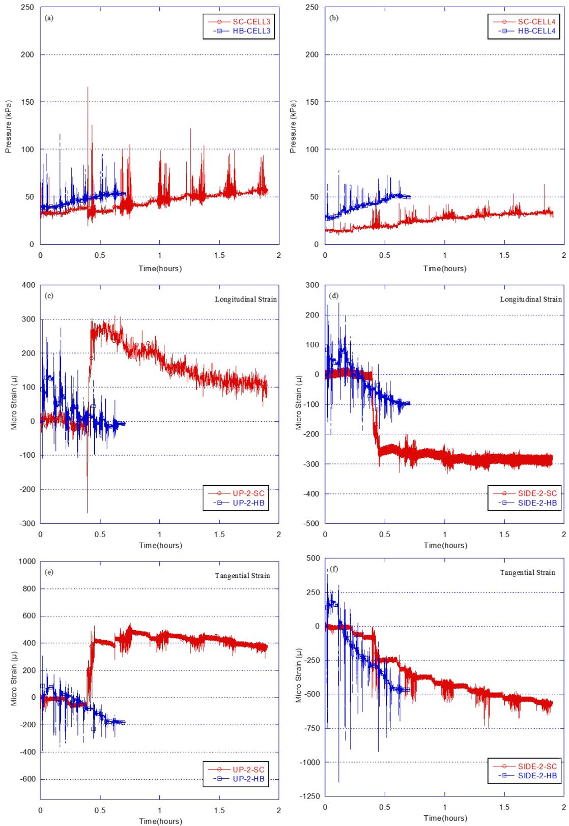
**Figure 5.4 Comparison of downward earth pressure and strains along pipe versus time between Test SC-4 and Test HB-16 (HDPE drainage pipe)**
