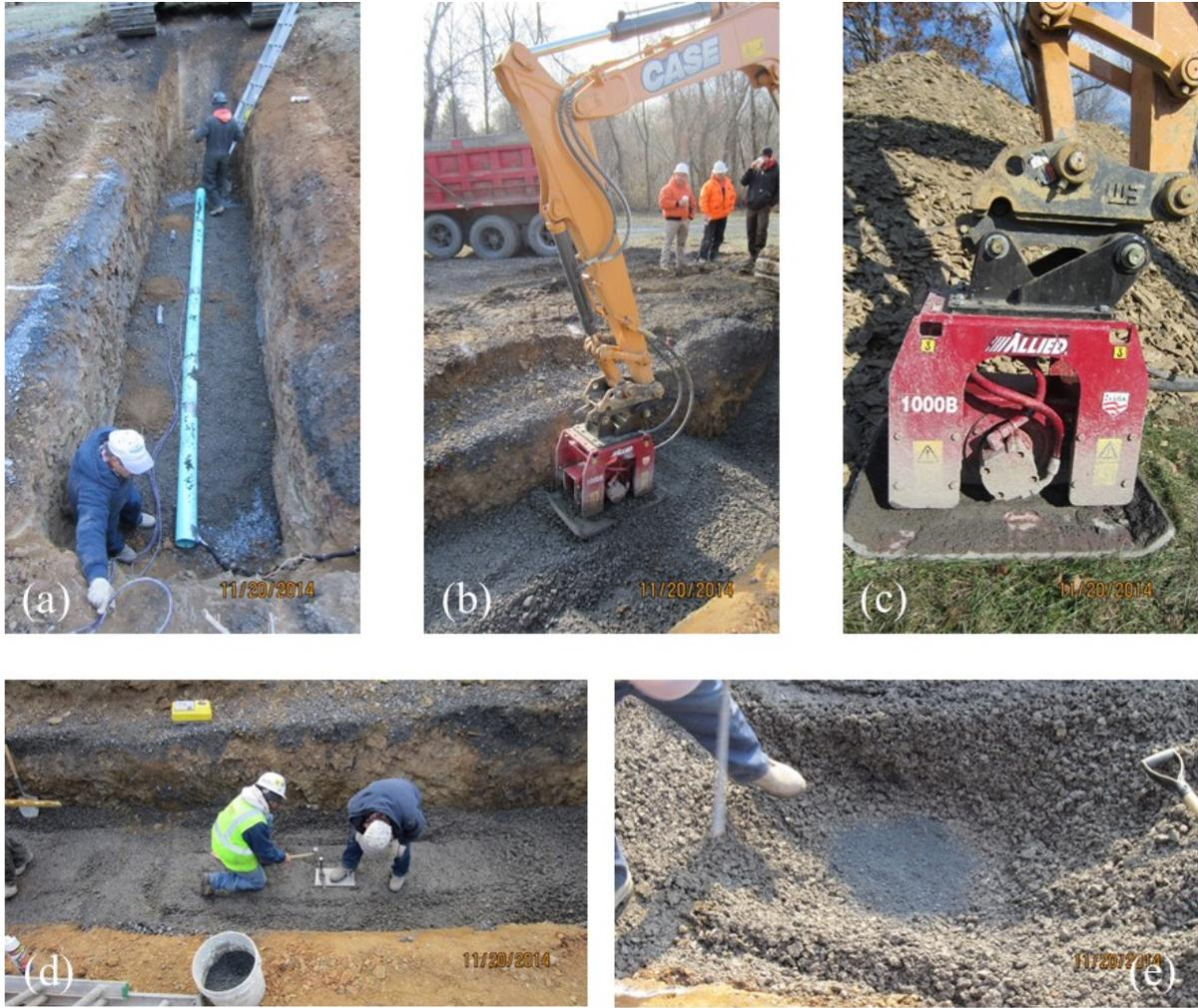
**Figure 4.14** Photos showing various stages of field test: a) placement of pressure cells on side along mid elevation of pipe; b) compaction using a hydraulic plate compactor; c) model of hydraulic plate compactor used: Applied 1000B; d) nuclear density gauge testing on a compacted surface; e) fine material is used to create a smooth surface in a scraped area for nuclear density gauge testing
