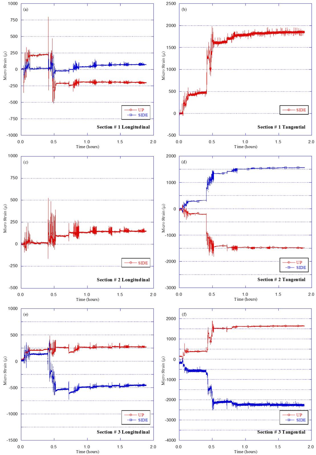
**Figure 3.12 Strains along pipe versus time for Test SC-2 (SDR-35 pipe in 2A aggregates)**
