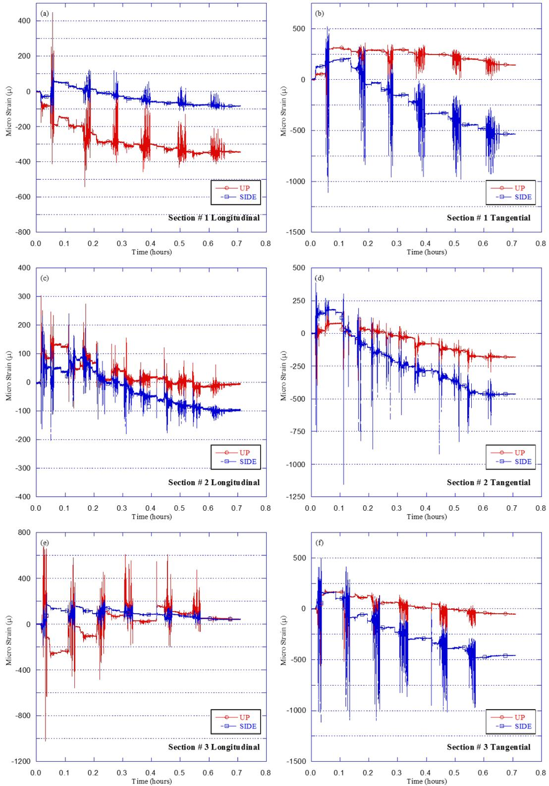
**Figure 4.44 Strains along pipe versus time for Test HB-16 (HDPE drainage pipe)**
