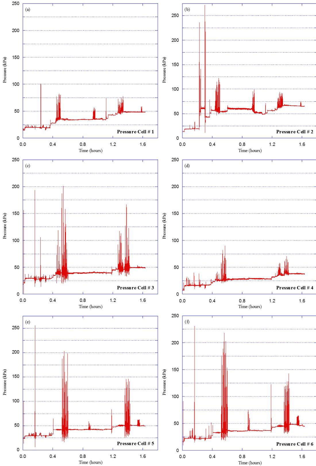
**Figure 4.15 Downward earth pressures versus time for Test HB-5 (SDR-35 pipe in 2A aggregates)**
