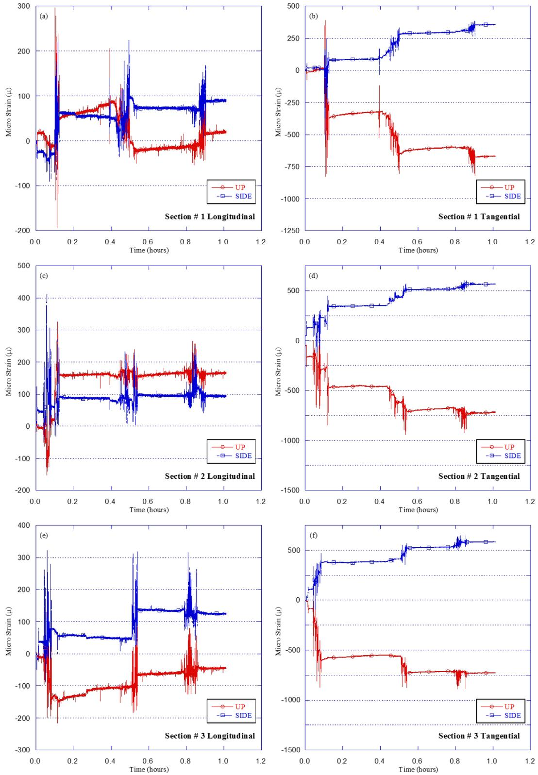
**Figure 4.7** Strains along pipe versus time for Test HB-2 (SDR-35 pipe in 2B stone)
