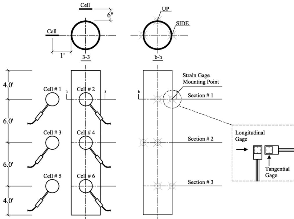
**Figure 3.19 Detailed view of instrumentation for 18-inch diameter HDPE drainage pipe (not to scale)**
