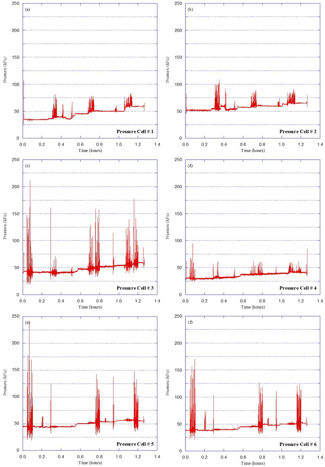
**Figure 4.17 Downward earth pressures versus time for Test HB-6 (SDR-35 pipe in 2A aggregates)**
