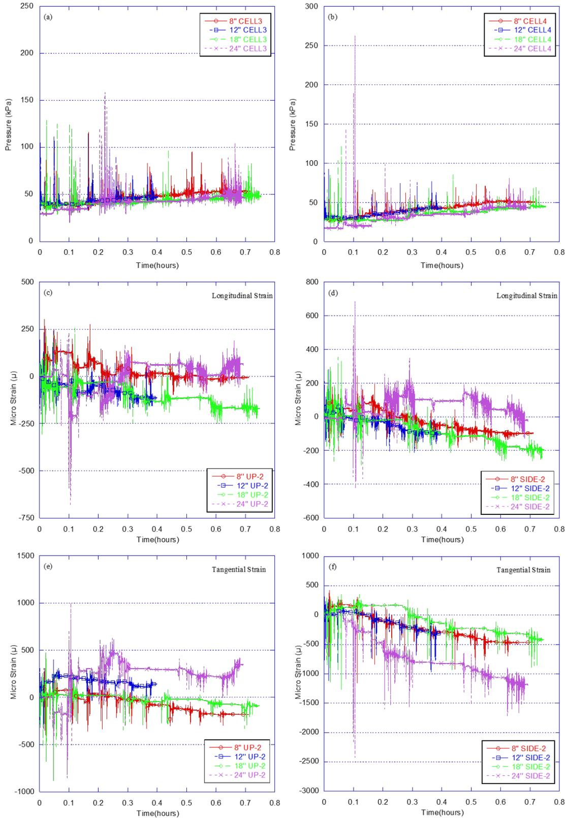
**Figure 5.8 Effect of lift thickness on downward earth pressure and strains along pipe versus time for HDPE drainage pipe**
