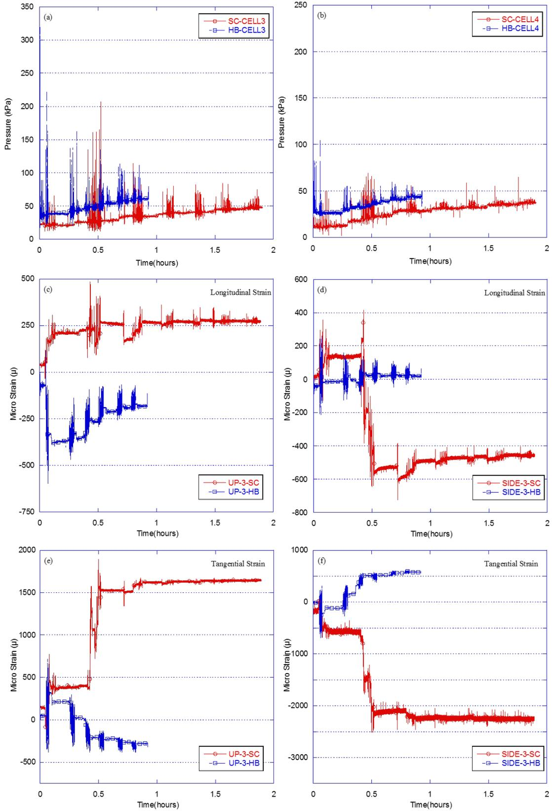
**Figure 5.2 Comparison of downward earth pressure and strains along pipe versus time between Test SC-2 and Test HB-8 (SDR-35 pipe in 2A aggregates)**
