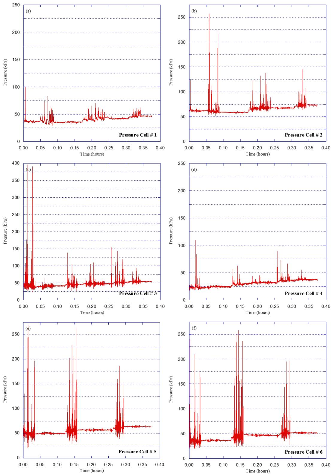
**Figure 4.30 Downward earth pressures versus time for Test HB-11 (reinforced concrete pipe)**
