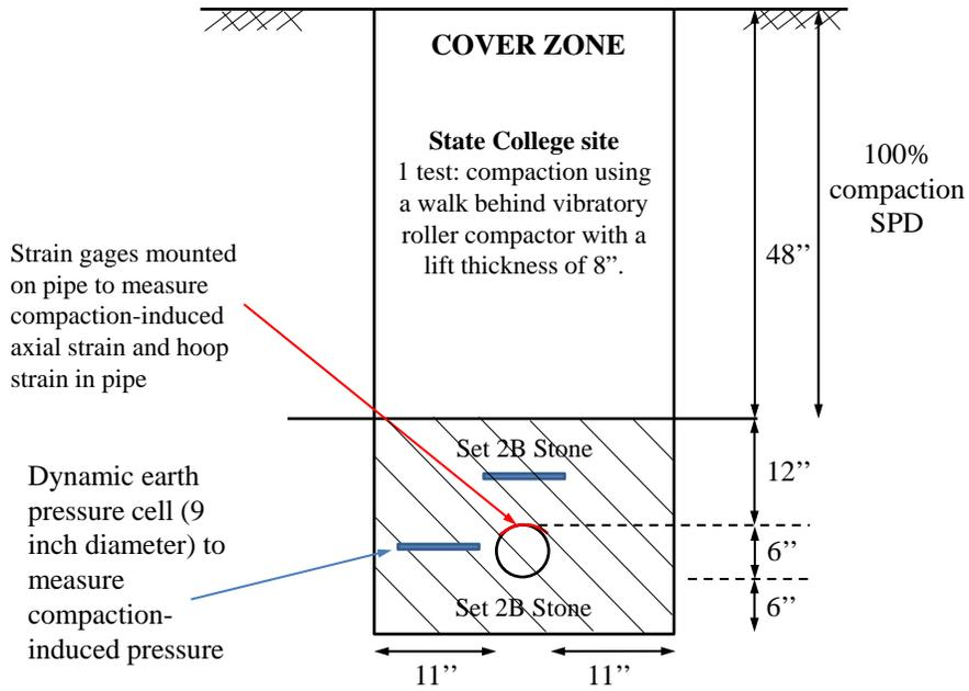
**Figure 3.1 Cross-sectional view of trench and instrumentation for 6-inch diameter SDR-35 pipe in 2B stone (not to scale)**
