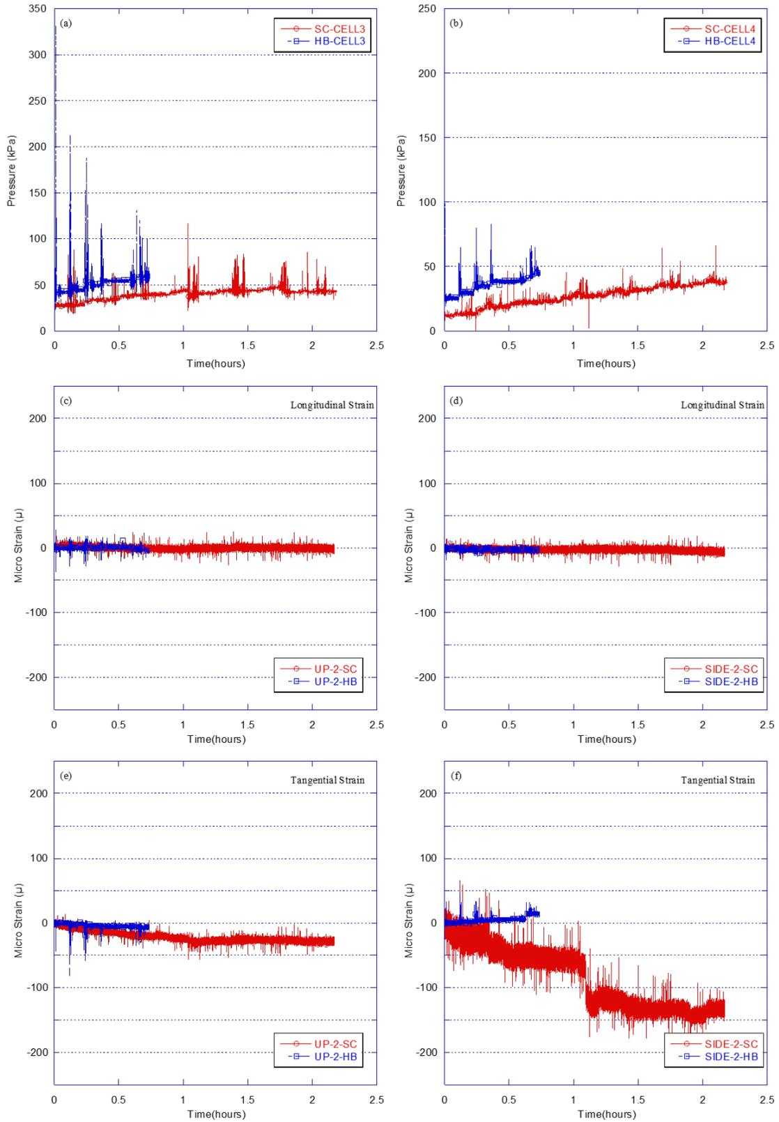
**Figure 5.3 Comparison of downward earth pressure and strains along pipe versus time between Test SC-3 and Test HB-12 (reinforced concrete pipe)**
