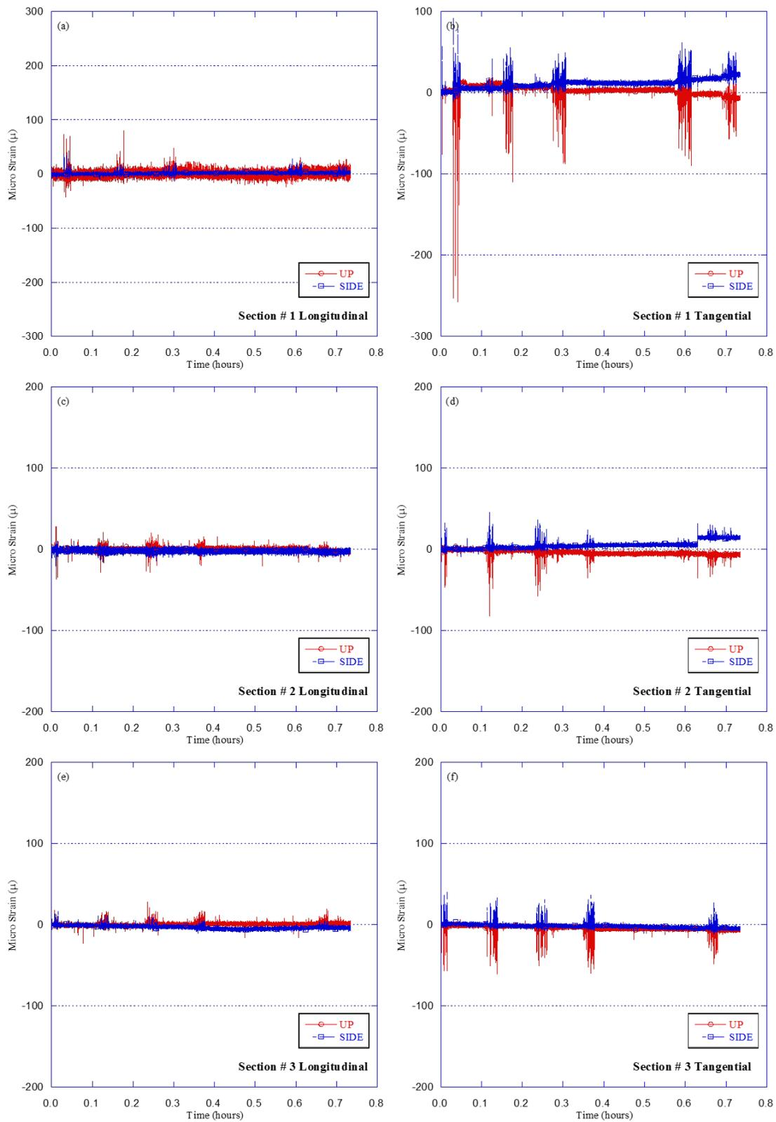
**Figure 4.33 Strains along pipe versus time for Test HB-12 (reinforced concrete pipe)**
