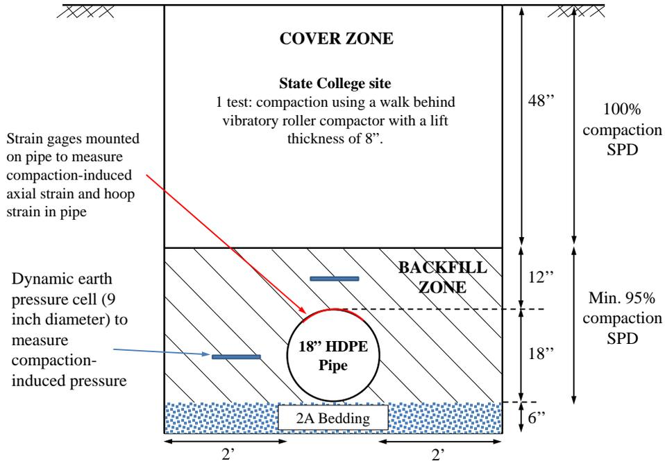
**Figure 3.18 Cross-sectional view of trench and instrumentation for 18-inch diameter HDPE drainage pipe (not to scale)**
