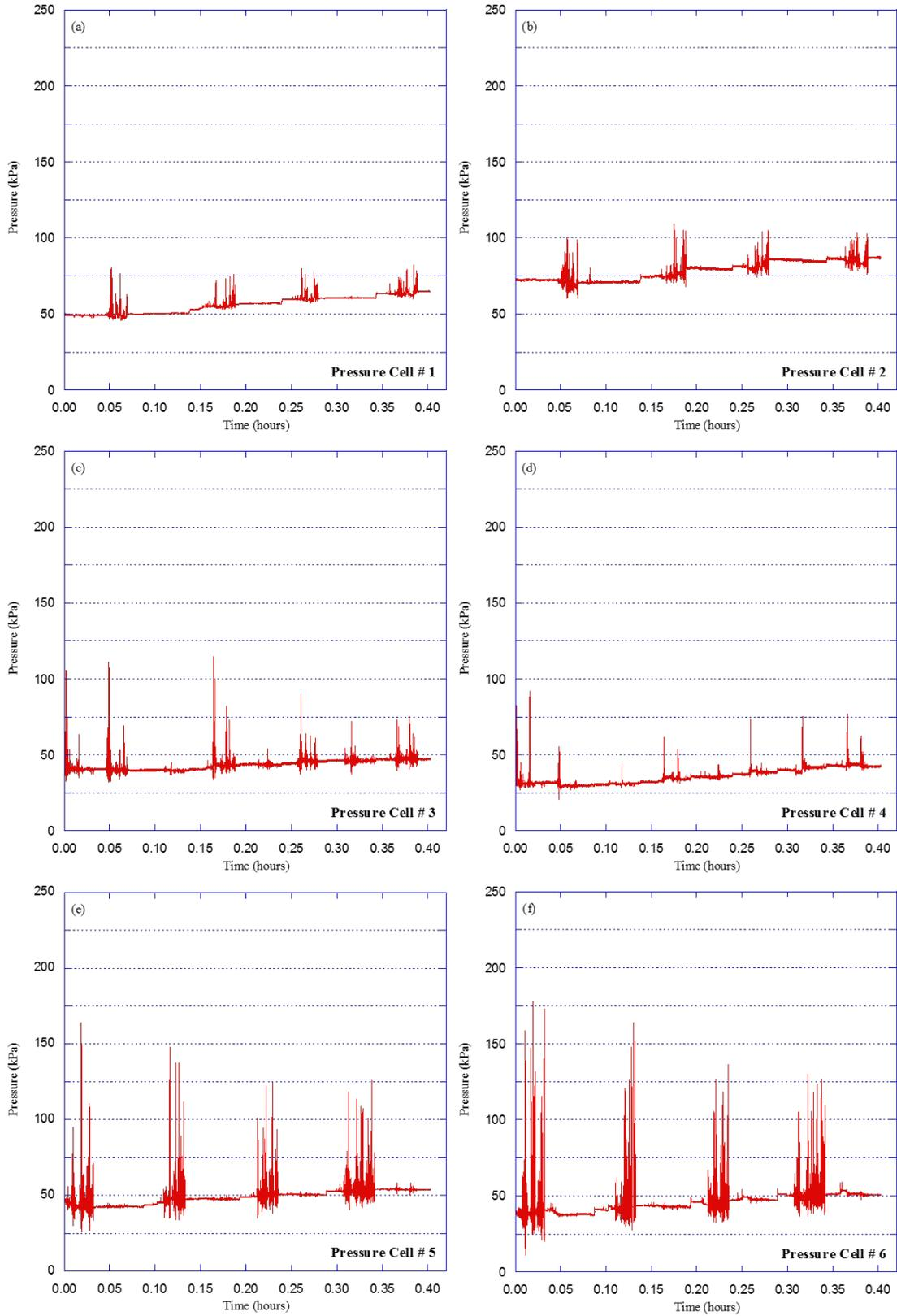
**Figure 4.41 Downward earth pressures versus time for Test HB-15 (HDPE drainage pipe)**
