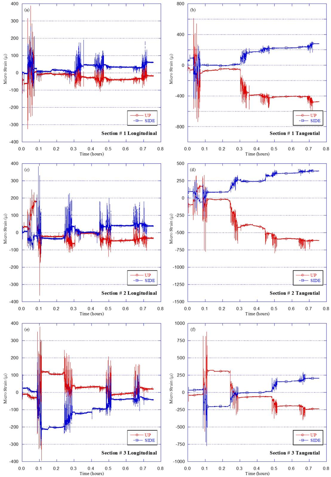
**Figure 4.9** Strains along pipe versus time for Test HB-3 (SDR-35 pipe in 2B stone)
