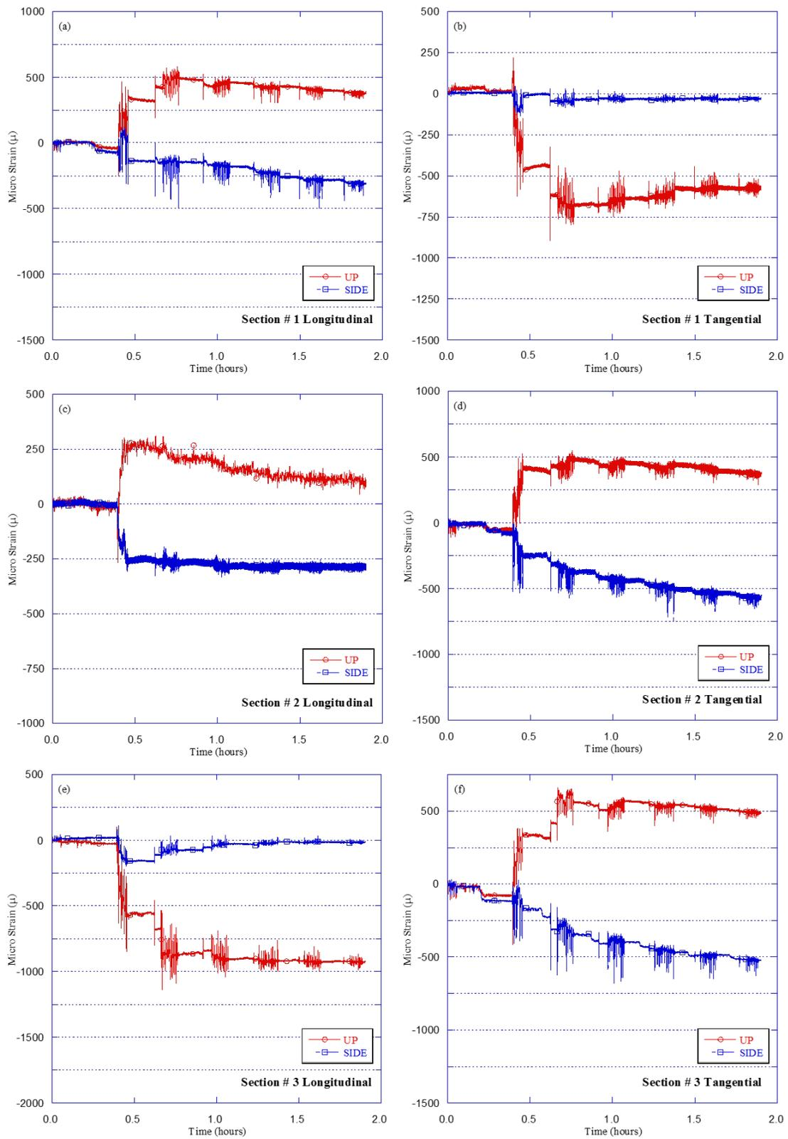
**Figure 3.22 Strains along pipe versus time for Test SC-4 (HDPE drainage pipe)**
