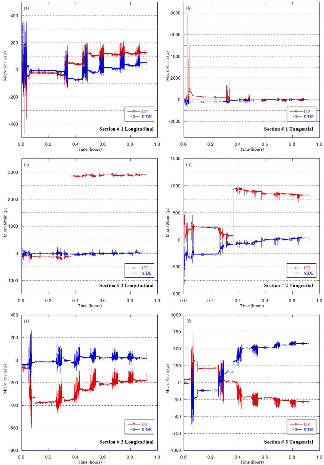
**Figure 4.22 Strains along pipe versus time for Test HB-8 (SDR-35 pipe in 2A aggregates)**
