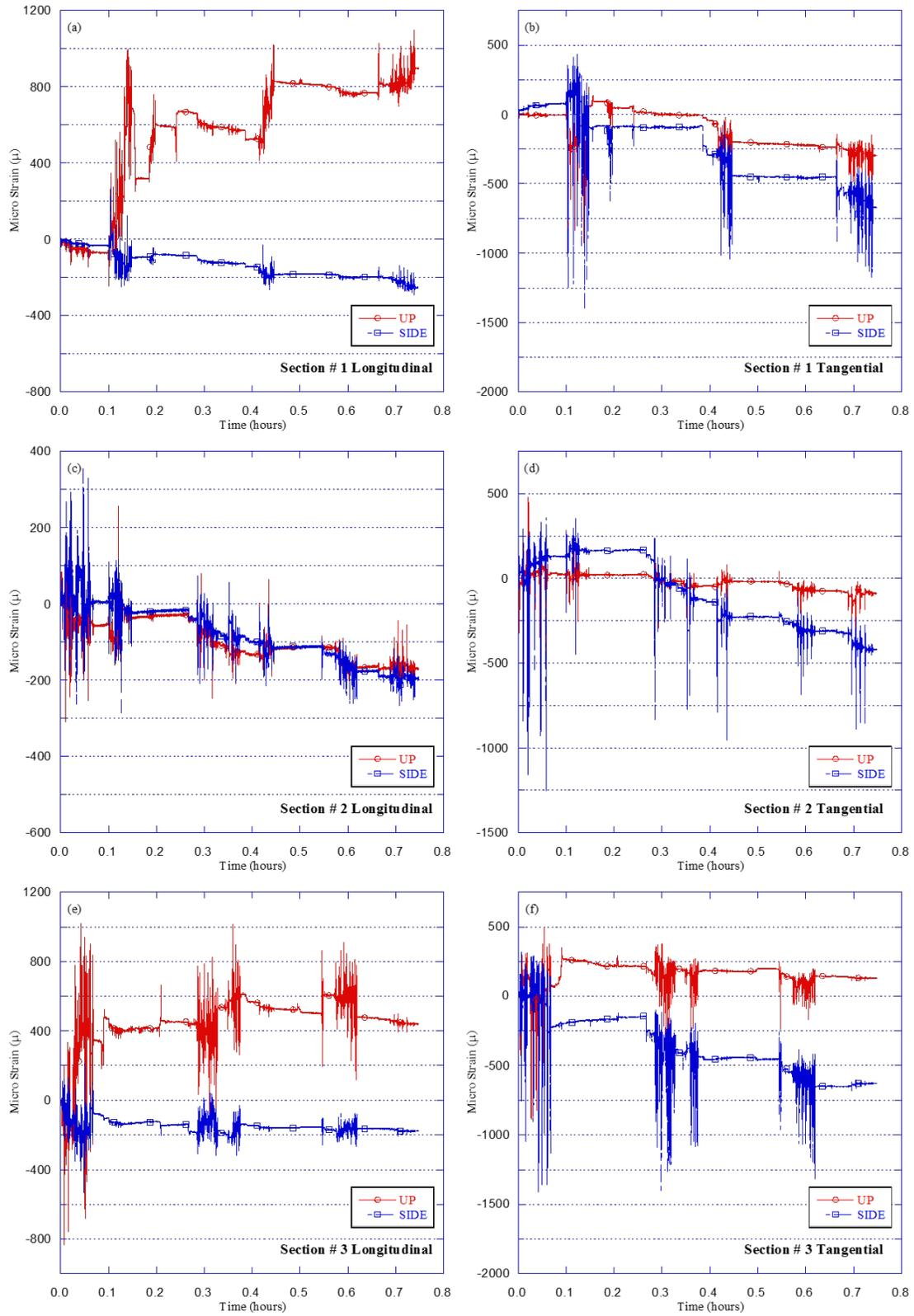
**Figure 4.40 Strains along pipe versus time for Test HB-14 (HDPE drainage pipe)**
