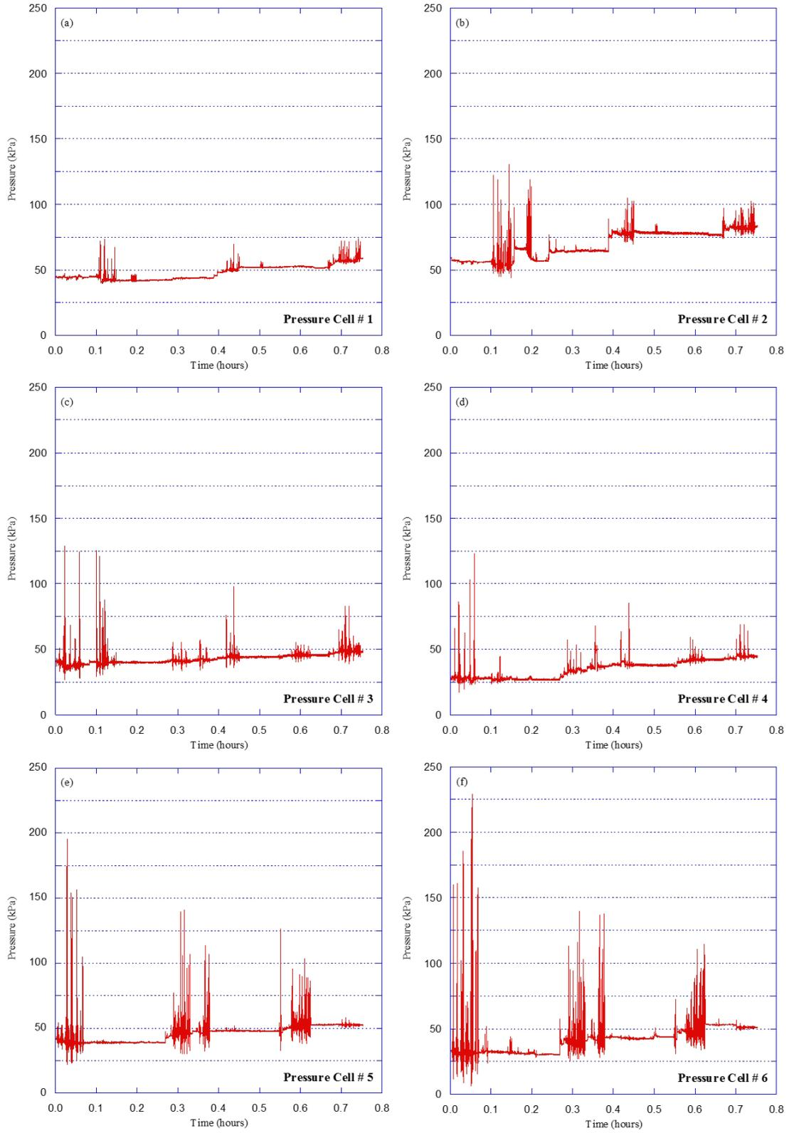
**Figure 4.39 Downward earth pressures versus time for Test HB-14 (HDPE drainage pipe)**
