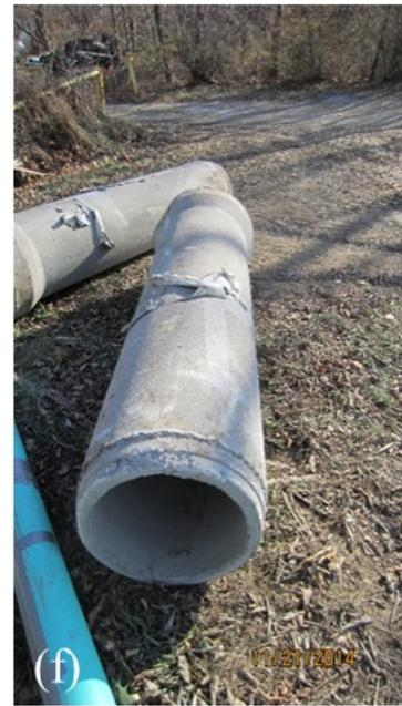
**Figure 4.25** Photos showing various stages of field test: a) AASHTO #8 bedding in trench; b) connecting concrete pipes in trench; c) dump fill materials into trench, both ends of concrete pipe covered by wood plate; d) compaction using a hydraulic plate compactor; e) excavating compacted fill materials; f) retrieved pipe after test
