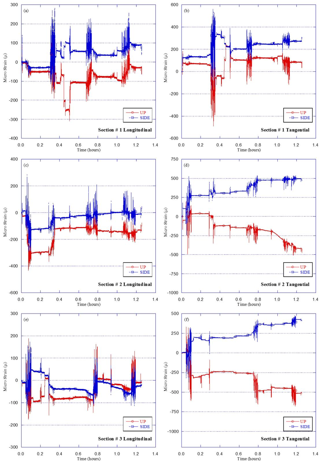
**Figure 4.18 Strains along pipe versus time for Test HB-6 (SDR-35 pipe in 2A aggregates)**
