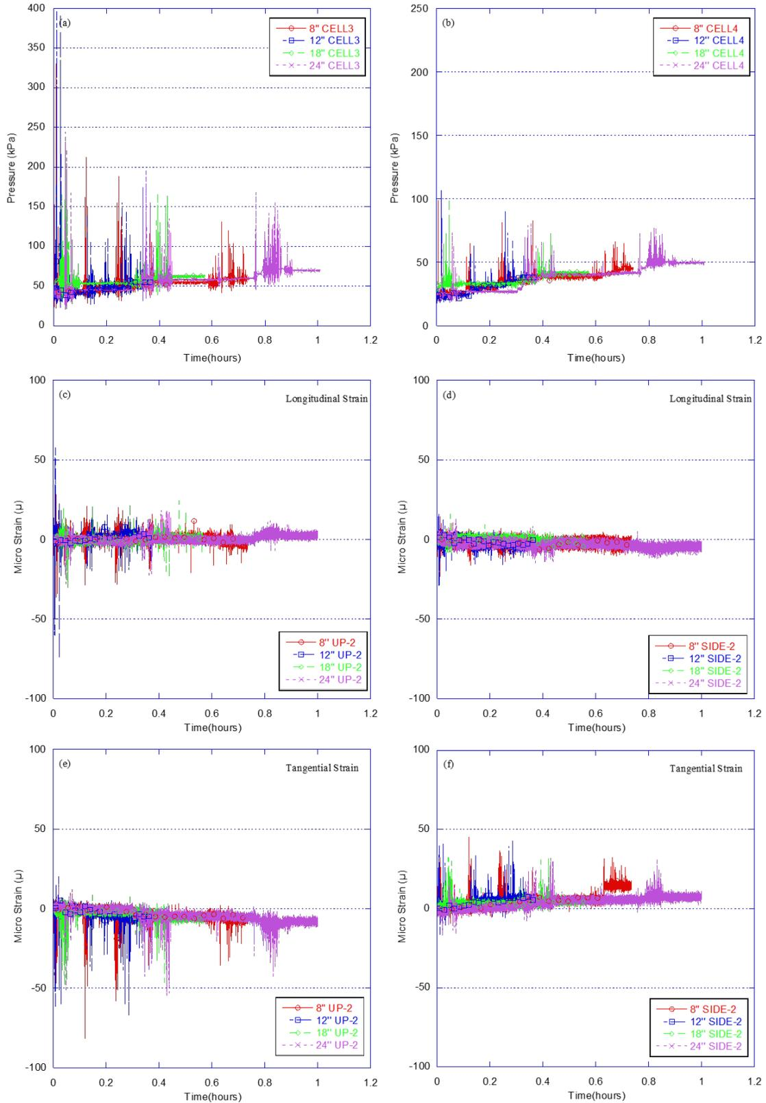
**Figure 5.7 Effect of lift thickness on downward earth pressure and strains along pipe versus time for reinforced concrete pipe**
