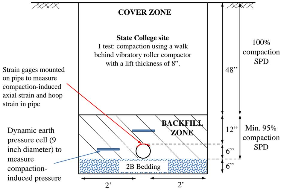
**Figure 3.8 Cross-sectional view of trench and instrumentation for 6-inch diameter SDR-35 pipe in 2A aggregates (not to scale)**
