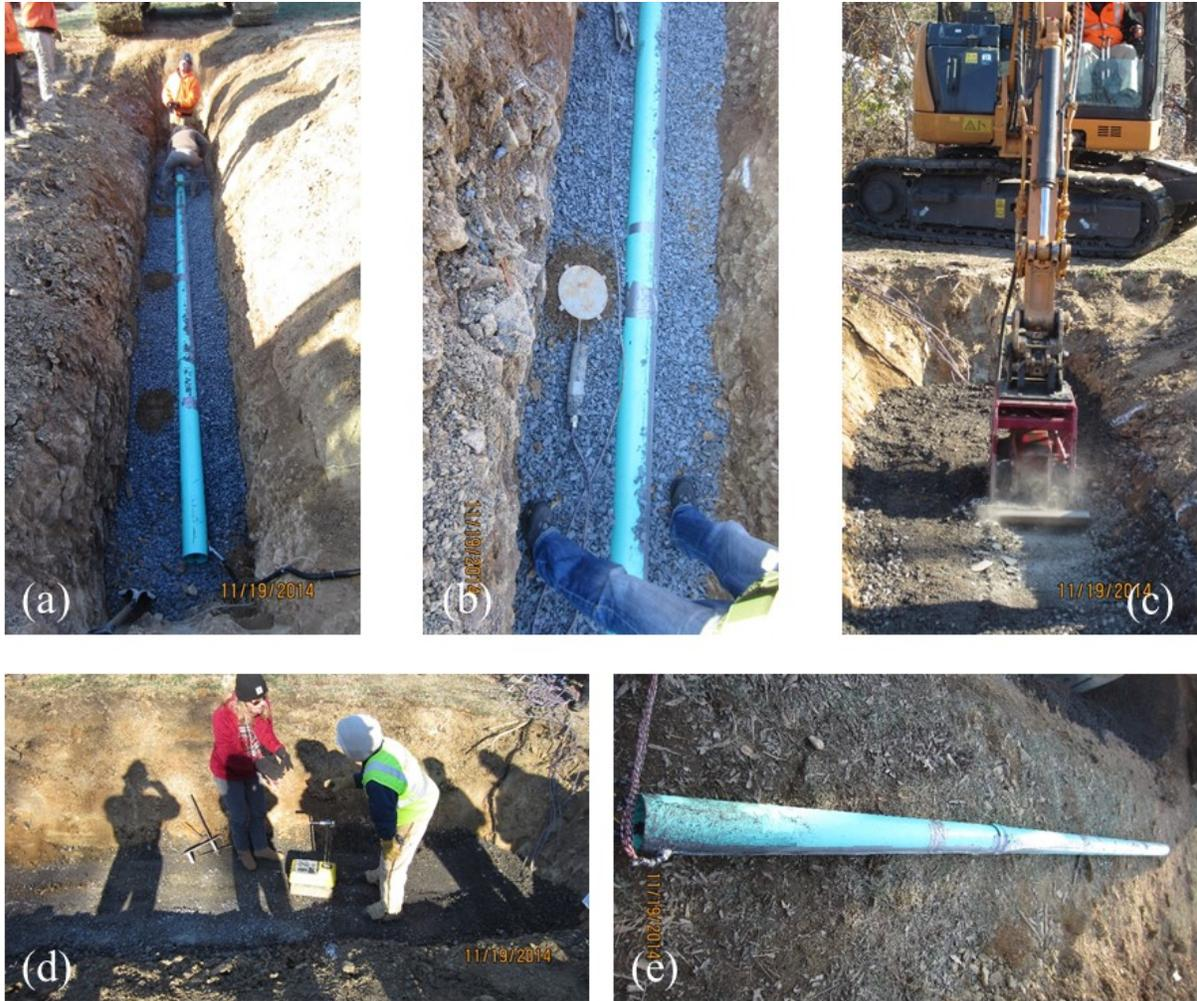
**Figure 4.3. Photos showing various stages of field test: a) 2B stone, pipe, and seating materials for placement of pressure cells; b) placement of a pressure cell on side along mid elevation of pipe; c) compaction using a hydraulic plate compactor; d) Ms. Robyn Myers giving instructions on nuclear density gauge testing; e) retrieved pipe after test**
