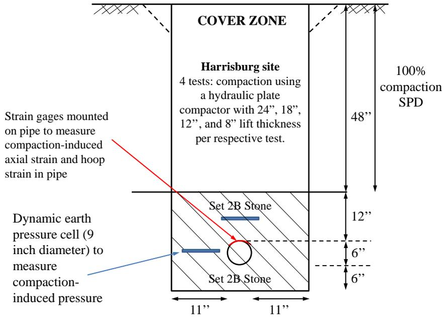
**Figure 4.1 Cross-sectional view of trench and instrumentation for 6-inch diameter SDR-35 pipe in 2B stone (not to scale)**
