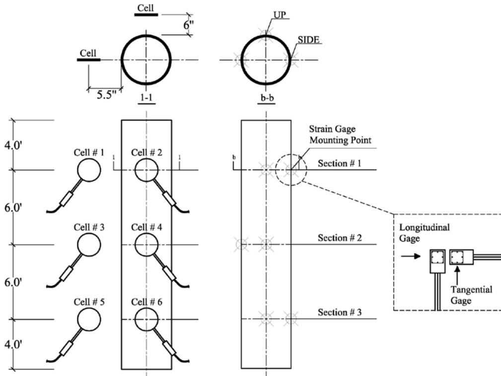
**Figure 4.2 Detailed view of instrumentation for 6-inch diameter SDR-35 pipe in 2B stone (not to scale)**
