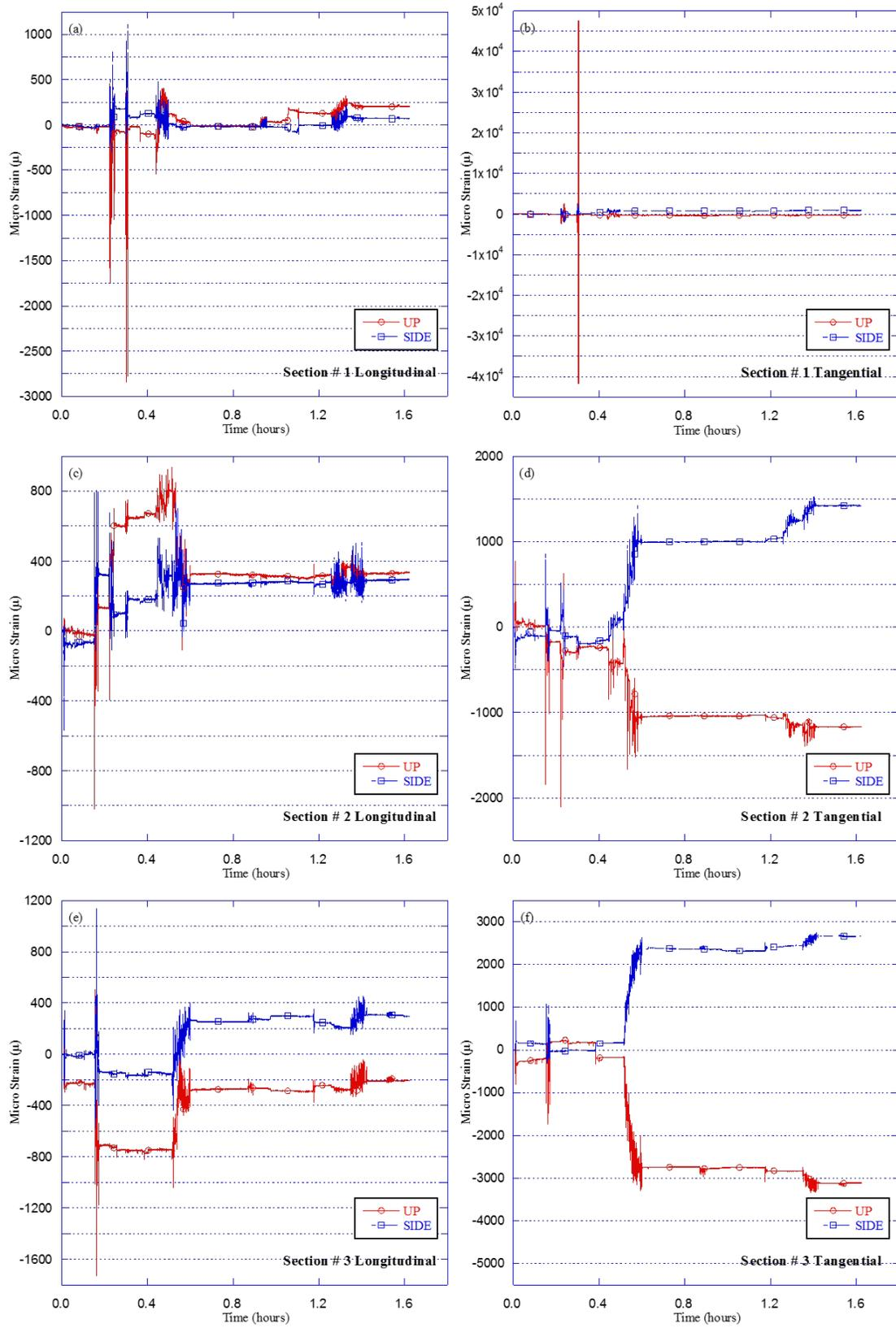
Figure 4.16 Strains along pipe versus time for Test HB-5 (SDR-35 pipe in 2A aggregates)
