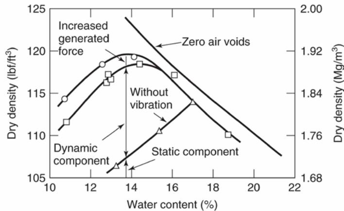
**Figure 2.1 Compaction results on 30-cm (12-inch) layers of silty sand, with and without vibration, using a 7,700-kg (17,000-lb) towed vibratory roller (after Parsons et al. 1962, as cited by Selig and Yoo 1977)**
