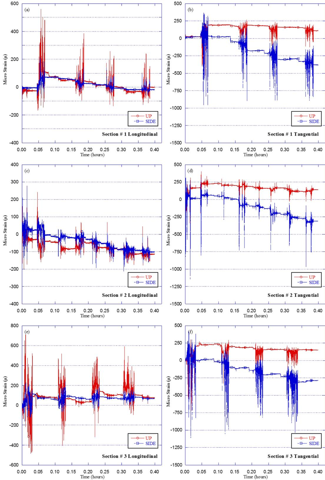
**Figure 4.42 Strains along pipe versus time for Test HB-15 (HDPE drainage pipe)**
