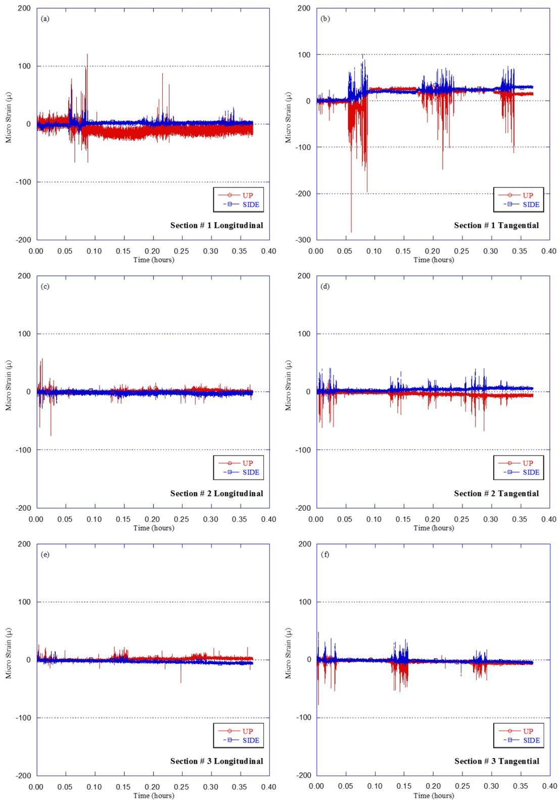
**Figure 4.31 Strains along pipe versus time for Test HB-11 (reinforced concrete pipe)**
