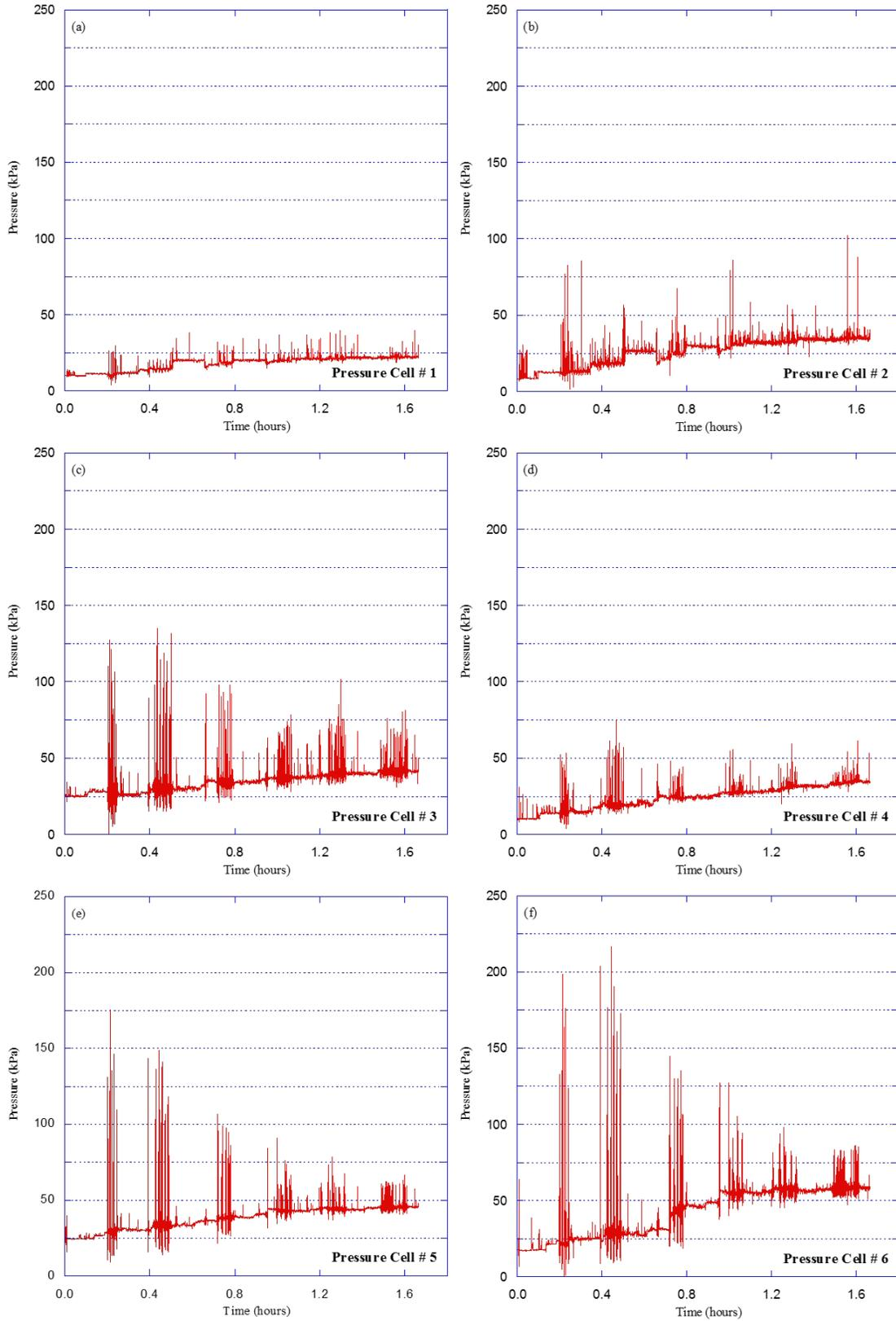
**Figure 3.6 Downward earth pressures versus time for Test SC-1 (SDR-35 pipe in 2B stone)**
