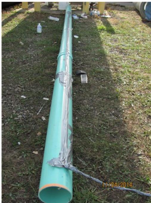
**Figure 3.3** A photo showing a fully instrumented 6-inch diameter SDR-35 pipe prior to placement
