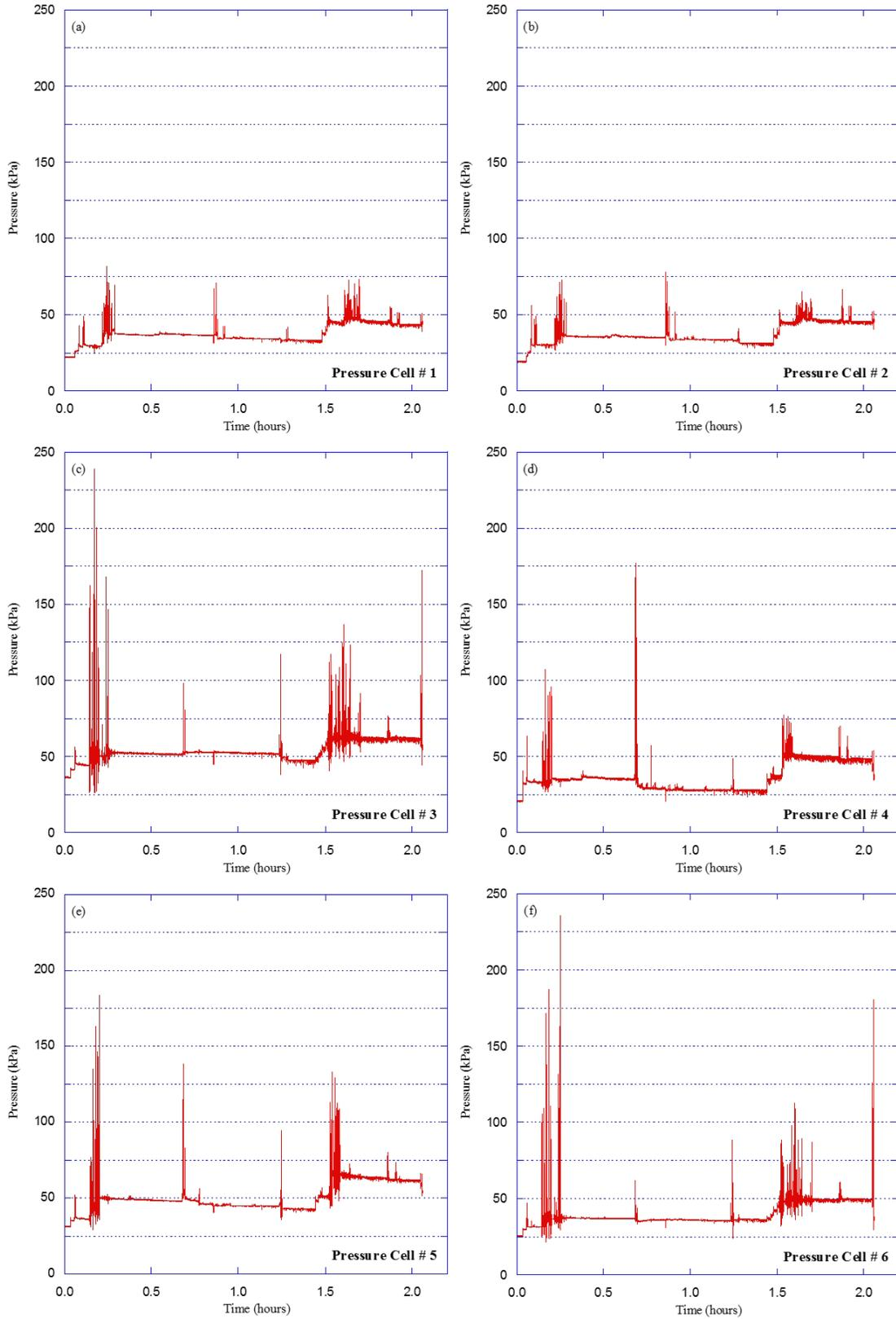
**Figure 4.4** Downward earth pressures versus time for Test HB-1 (SDR-35 pipe in 2B stone)
