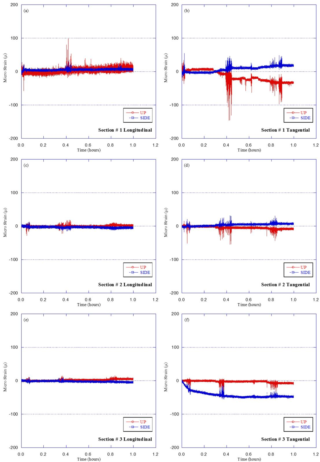
**Figure 4.27 Strains along pipe versus time for Test HB-9 (reinforced concrete pipe)**
