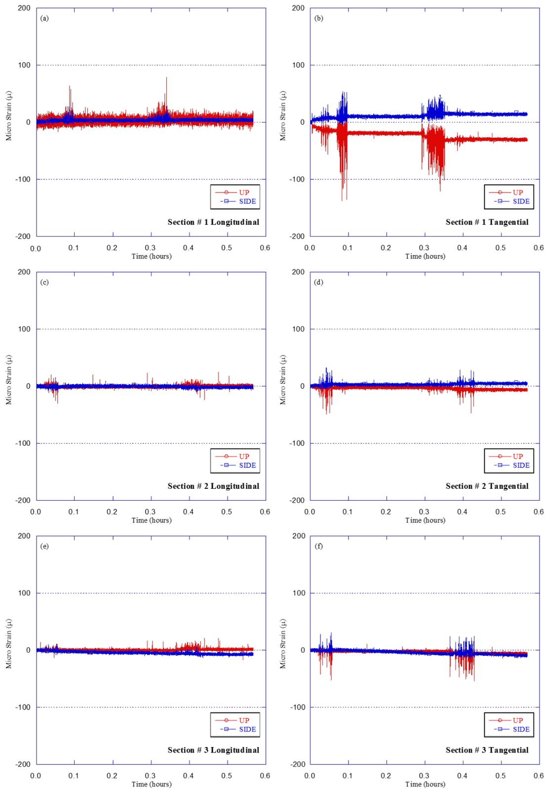
**Figure 4.29 Strains along pipe versus time for Test HB-10 (reinforced concrete pipe)**
