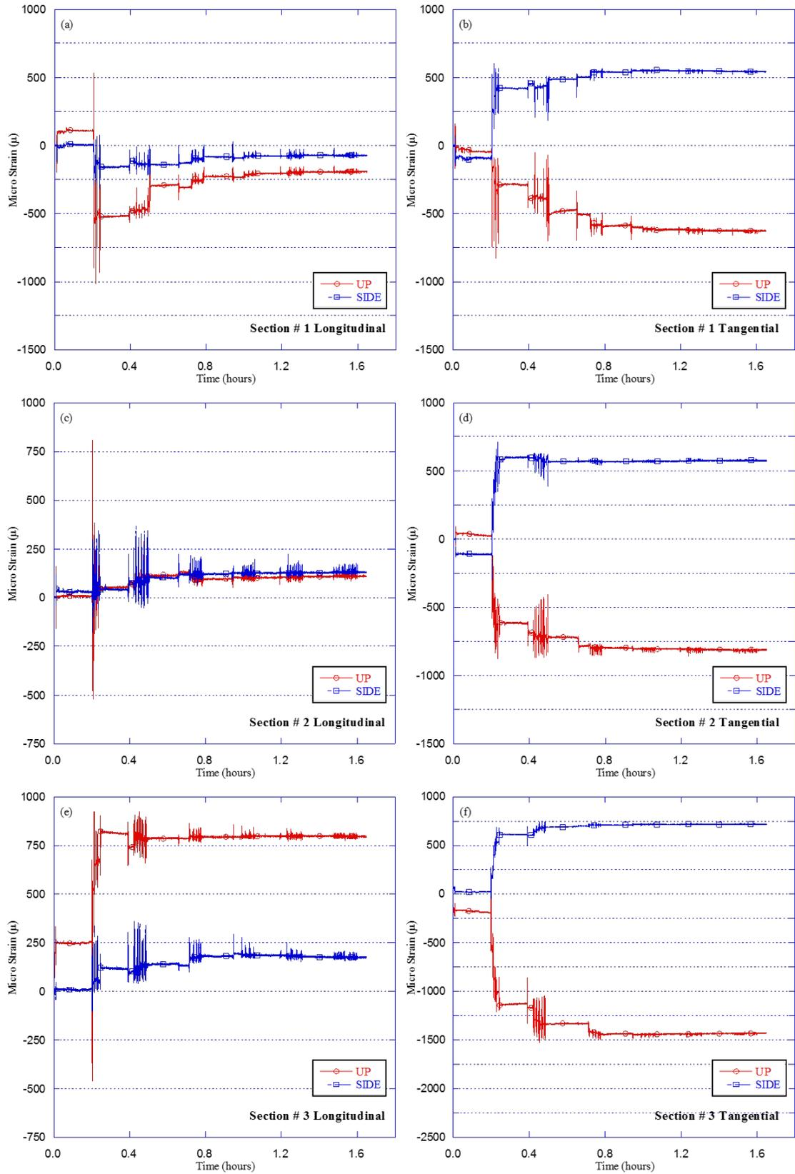
**Figure 3.7 Strains along pipe versus time for Test SC-1 (SDR-35 pipe in 2B stone)**
