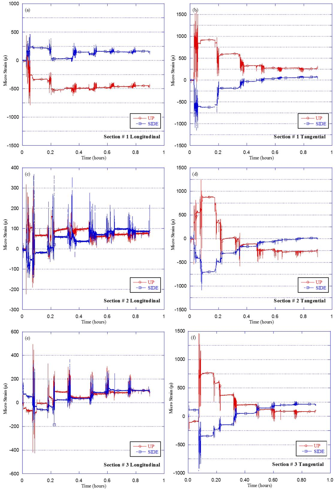
**Figure 4.11 Strains along pipe versus time for Test HB-4 (SDR-35 pipe in 2B stone)**
