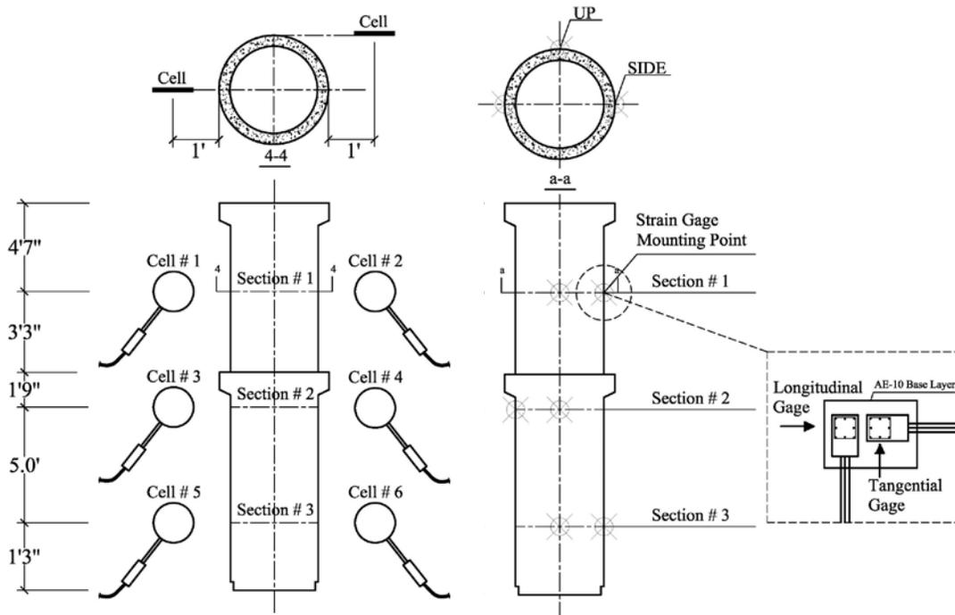
**Figure 4.24 Detailed view of instrumentation for 18-inch diameter reinforced concrete pipe (not to scale)**
