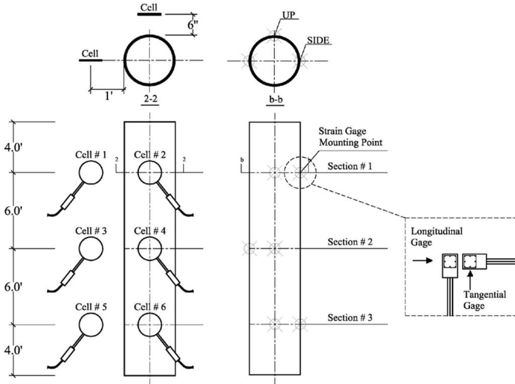
**Figure 4.13 Detailed view of instrumentation for 6-inch diameter SDR-35 pipe in 2A aggregates (not to scale)**
