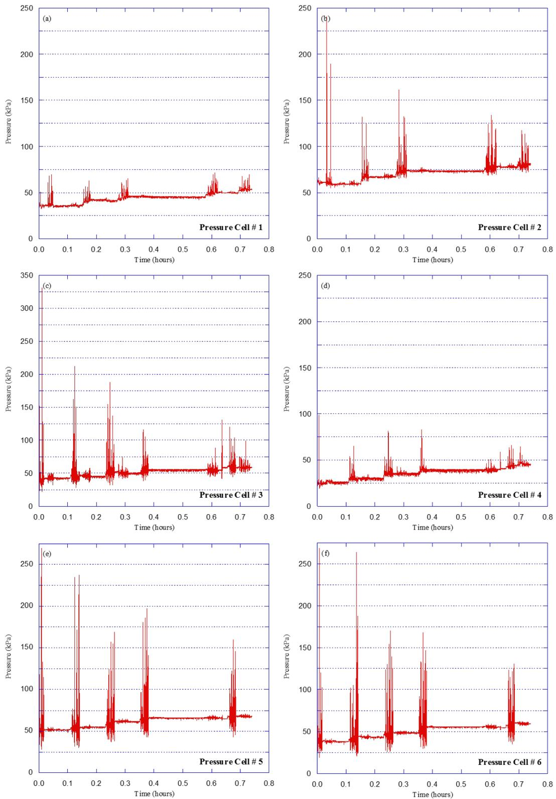
**Figure 4.32 Downward earth pressures versus time for Test HB-12 (reinforced concrete pipe)**
