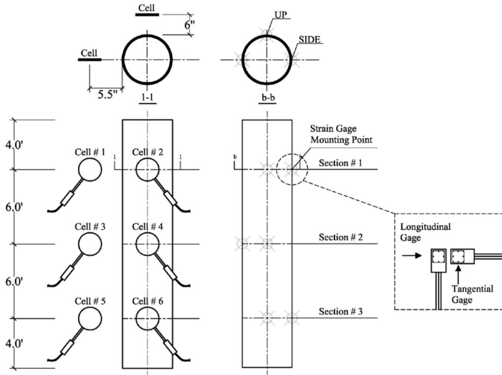
**Figure 3.2 Detailed view of instrumentation for 6-inch diameter SDR-35 pipe in 2B stone (not to scale)**
