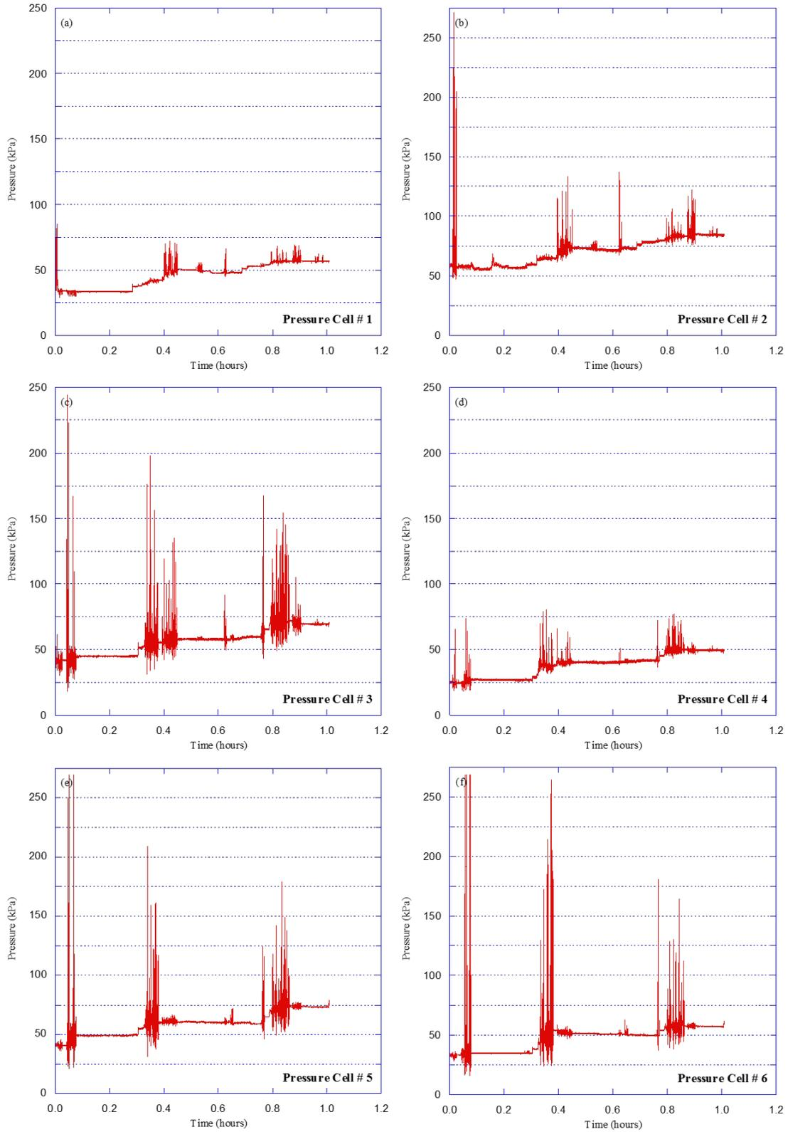
**Figure 4.26 Downward earth pressures versus time for Test HB-9 (reinforced concrete pipe)**
