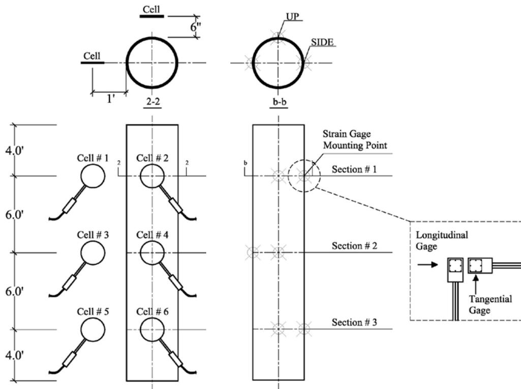
**Figure 3.9 Detailed view of instrumentation for 6-inch diameter SDR-35 pipe in 2A aggregates (not to scale)**
