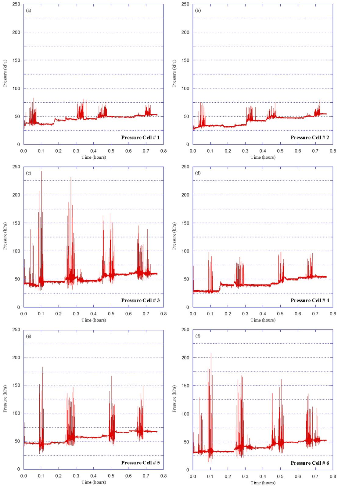
**Figure 4.8 Downward earth pressures versus time for Test HB-3 (SDR-35 pipe in 2B stone)**
