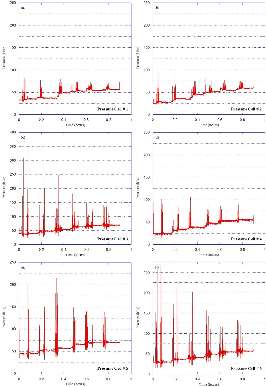
**Figure 4.10 Downward earth pressures versus time for Test HB-4 (SDR-35 pipe in 2B stone)**
