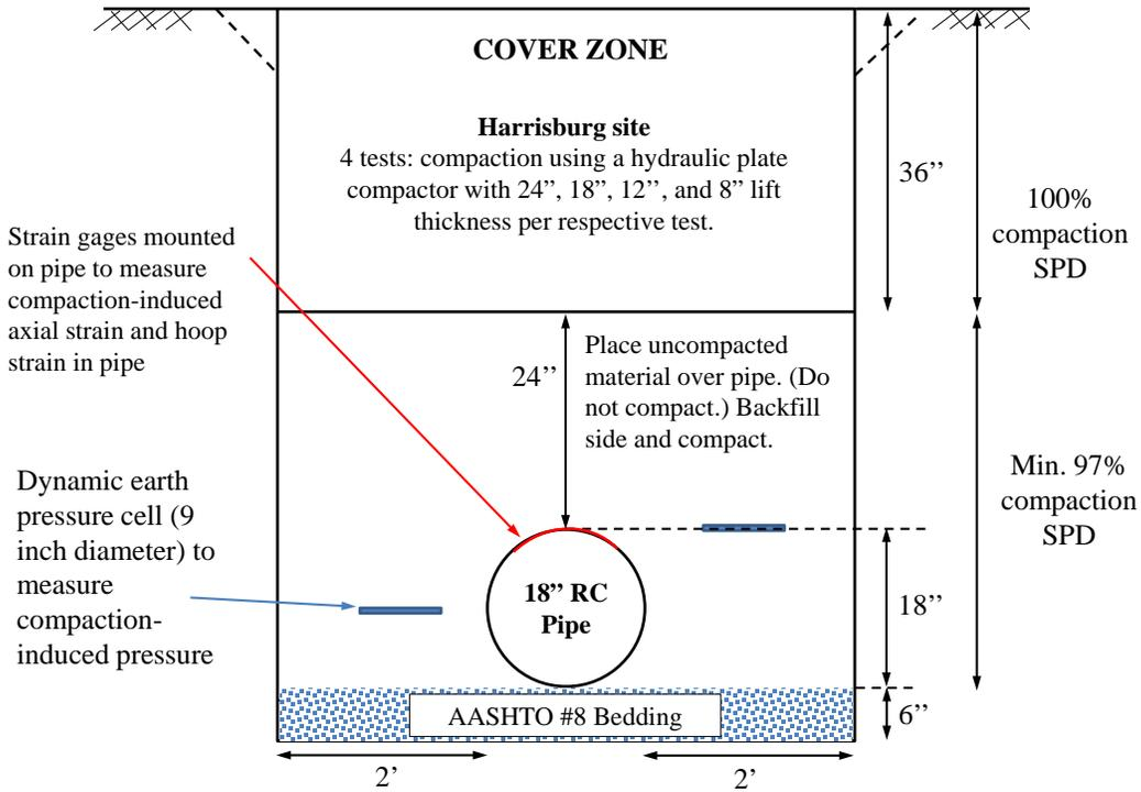
**Figure 4.23 Cross-sectional view of trench and instrumentation for 18-inch diameter reinforced concrete pipe (not to scale)**
