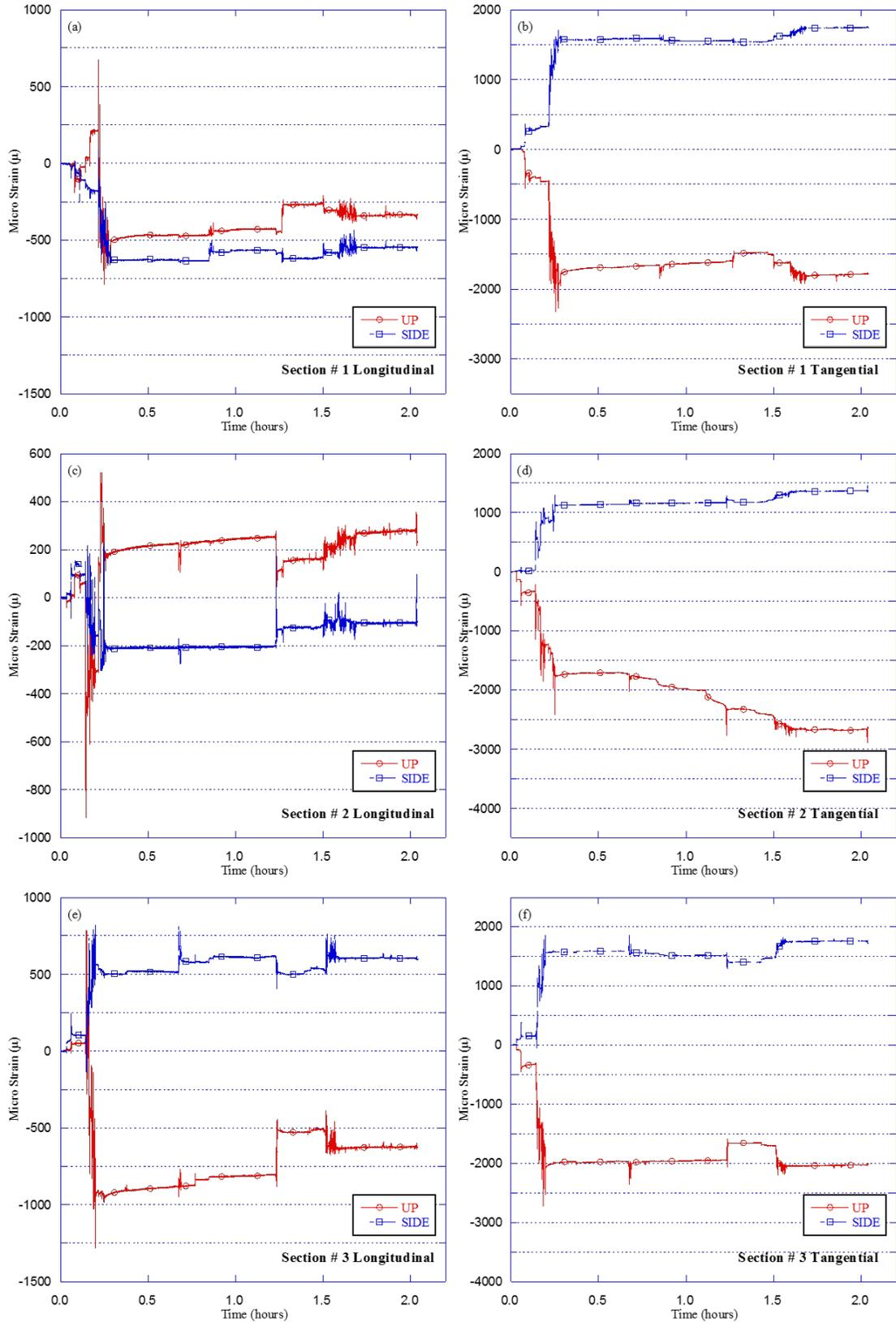
**Figure 4.5 Strains along pipe versus time for Test HB-1 (SDR-35 pipe in 2B stone)**
