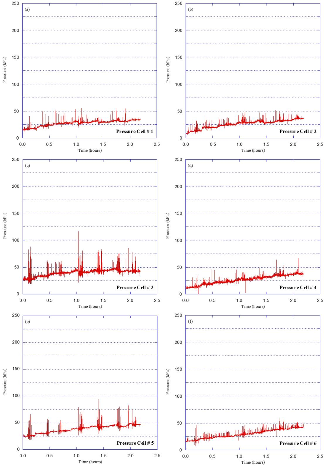
**Figure 3.16 Downward earth pressures versus time for Test SC-3 (reinforced concrete pipe)**
