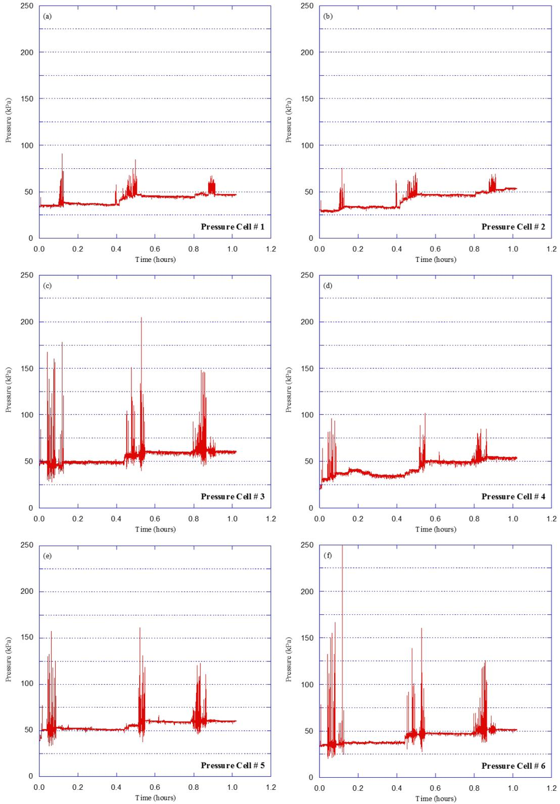
**Figure 4.6 Downward earth pressures versus time for Test HB-2 (SDR-35 pipe in 2B stone)**
