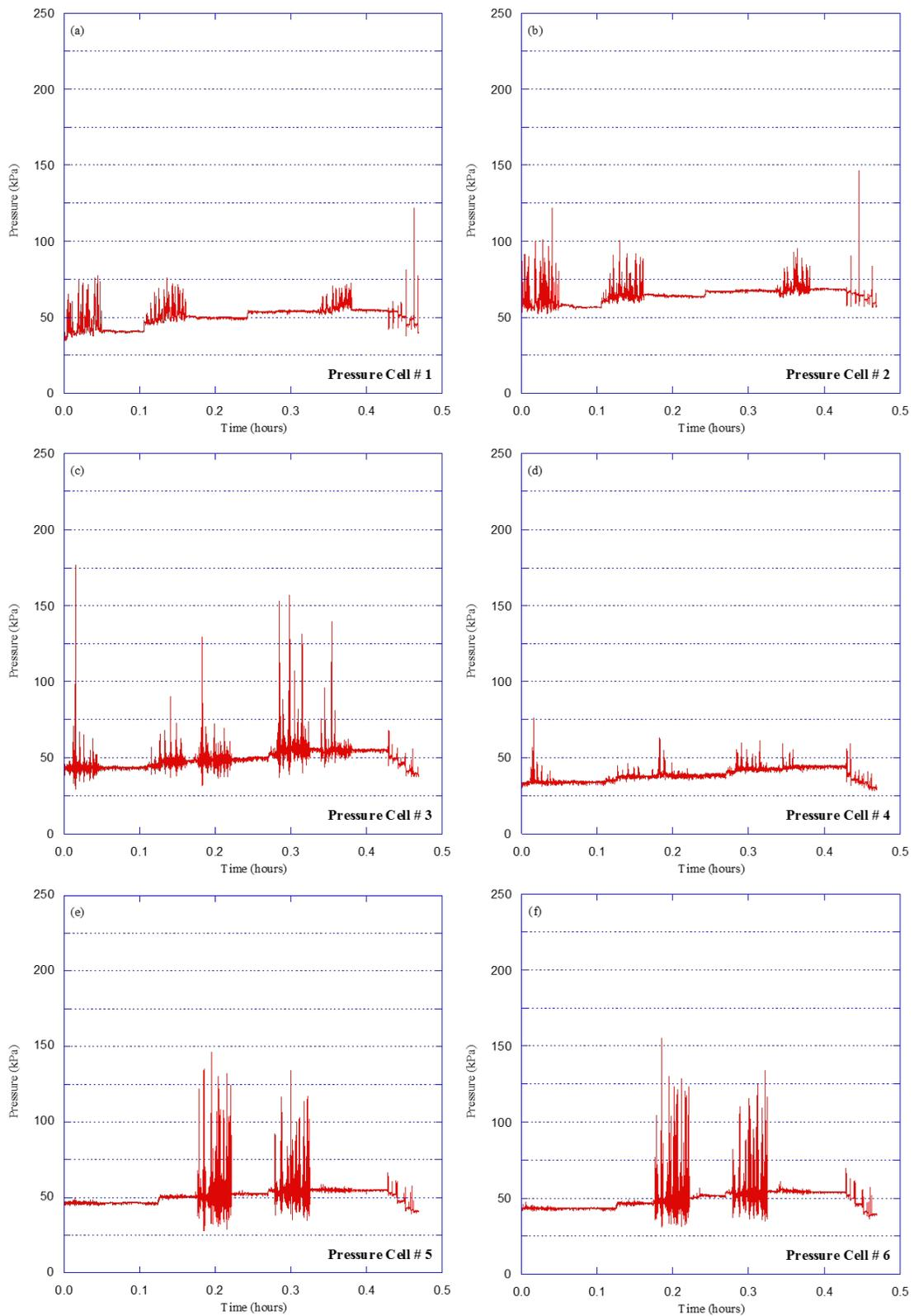
**Figure 4.19 Downward earth pressures versus time for Test HB-7 (SDR-35 pipe in 2A aggregates)**
