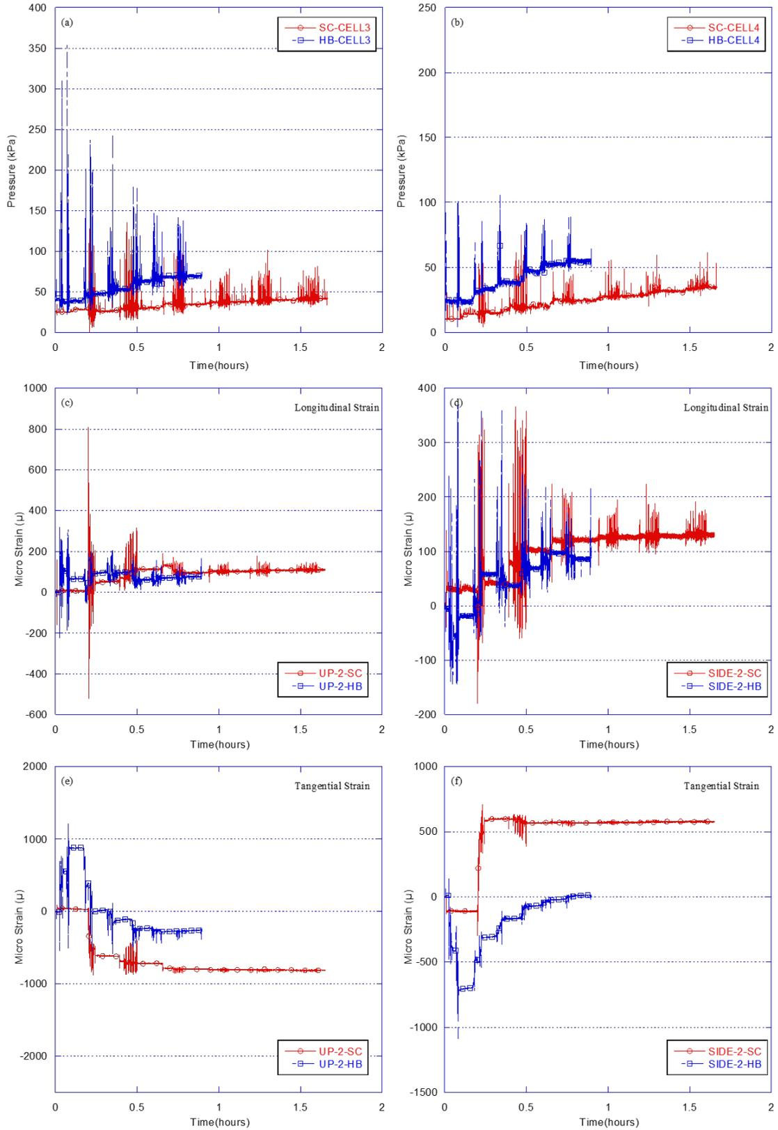
**Figure 5.1 Comparison of downward earth pressure and strains along pipe versus time between Test SC-1 and Test HB-4 (SDR-35 pipe in 2B stone)**
