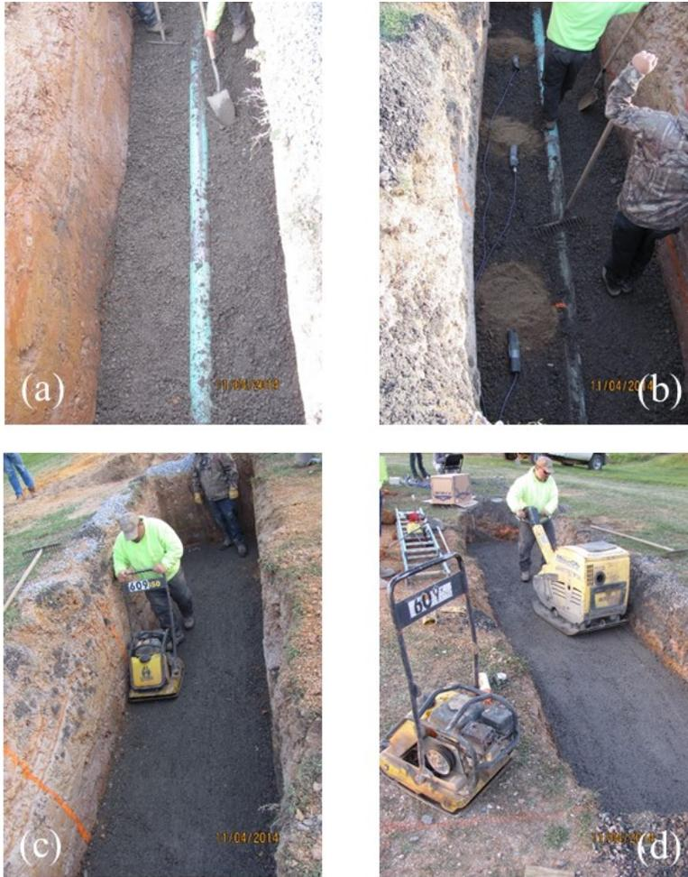
**Figure 3.10 Photos showing various stages of field test: a) add 2A aggregates to mid elevation of pipe; b) placement of pressure cells on side along mid elevation of pipe; c) compaction using a small tamper at top of backfill zone; d) compaction using a walk-behind vibratory roller compactor in cover zone**
