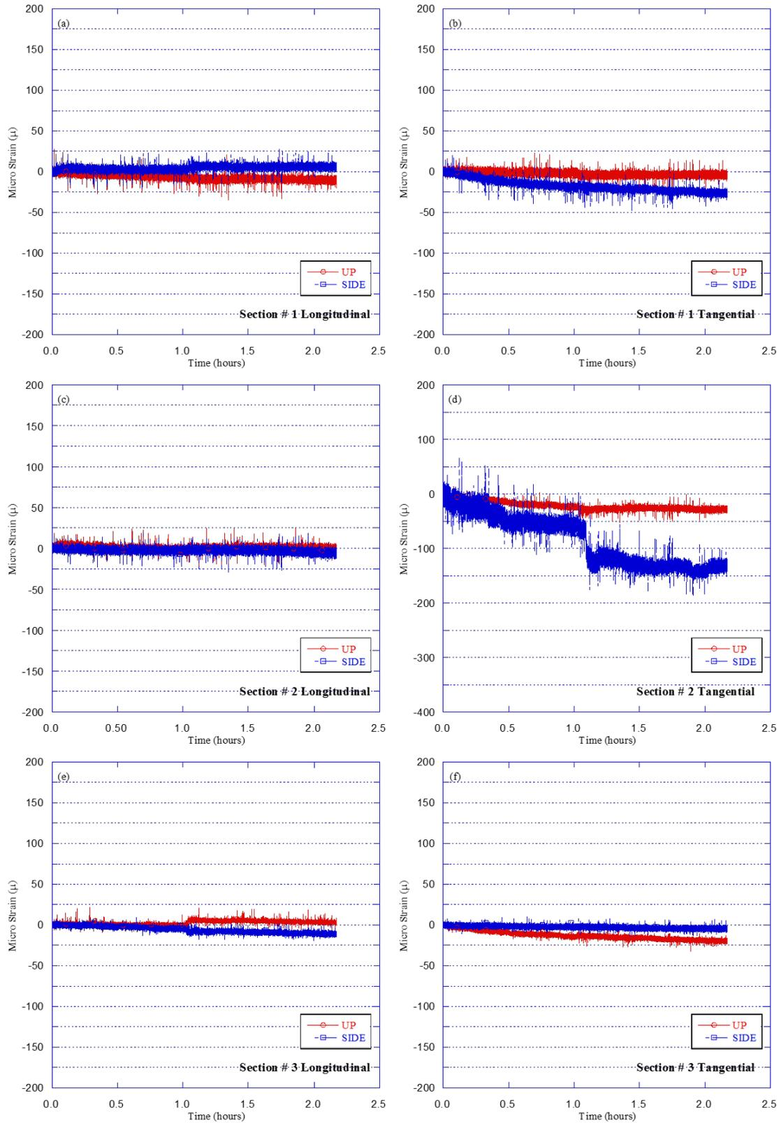
**Figure 3.17 Strains along pipe versus time for Test SC-3 (reinforced concrete pipe)**
